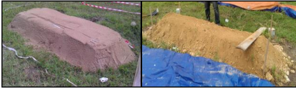
Fig. 1. Small model of soil trail embankment built up using sandy soil (left) and lateritic (right) soil.
