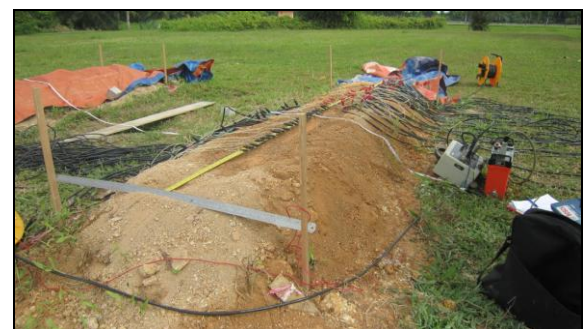
Fig. 3. Soil model 2 (lateritic soil) tested by 2D electrical resistivity imaging.
