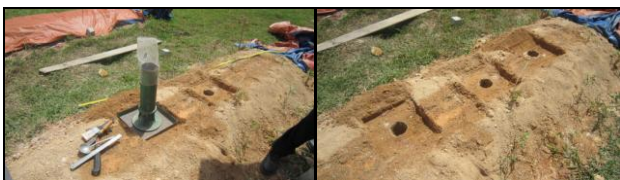
Fig. 4. Field density test using sand replacement method at lateritic soil model.
