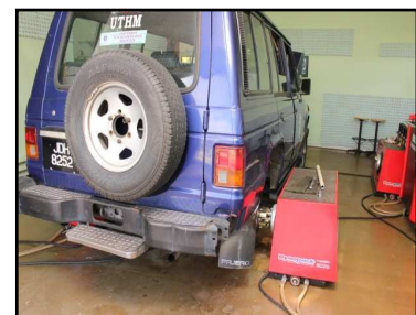
(b) Test vehicle and chassis dynamometer set up
