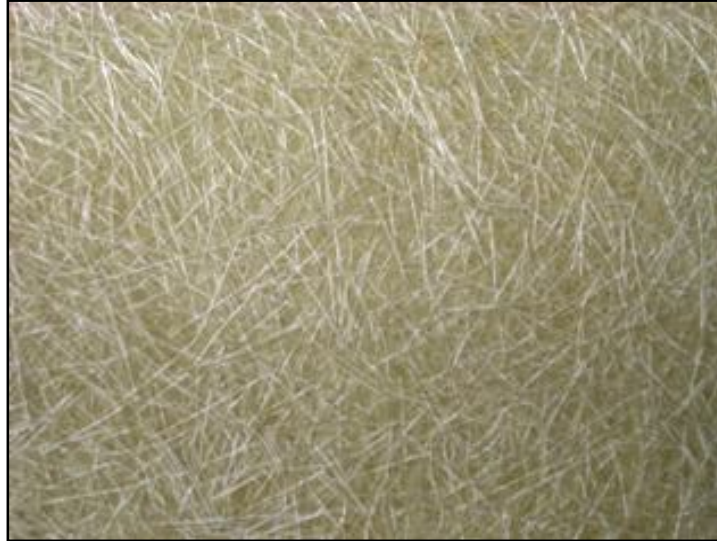
Figure 2.9: Chopped strand glass fibers.
