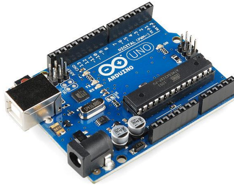
Figure 3.4: Arduino Uno R3 mainboard
