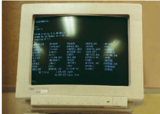
Figure 2.3 : Veiling reflection: the reflection of light is masking information on the screen.
