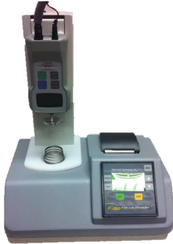
Figure 12 - Photography showing the Egg Force Reader that was used to evaluate egg shell breaking strength
