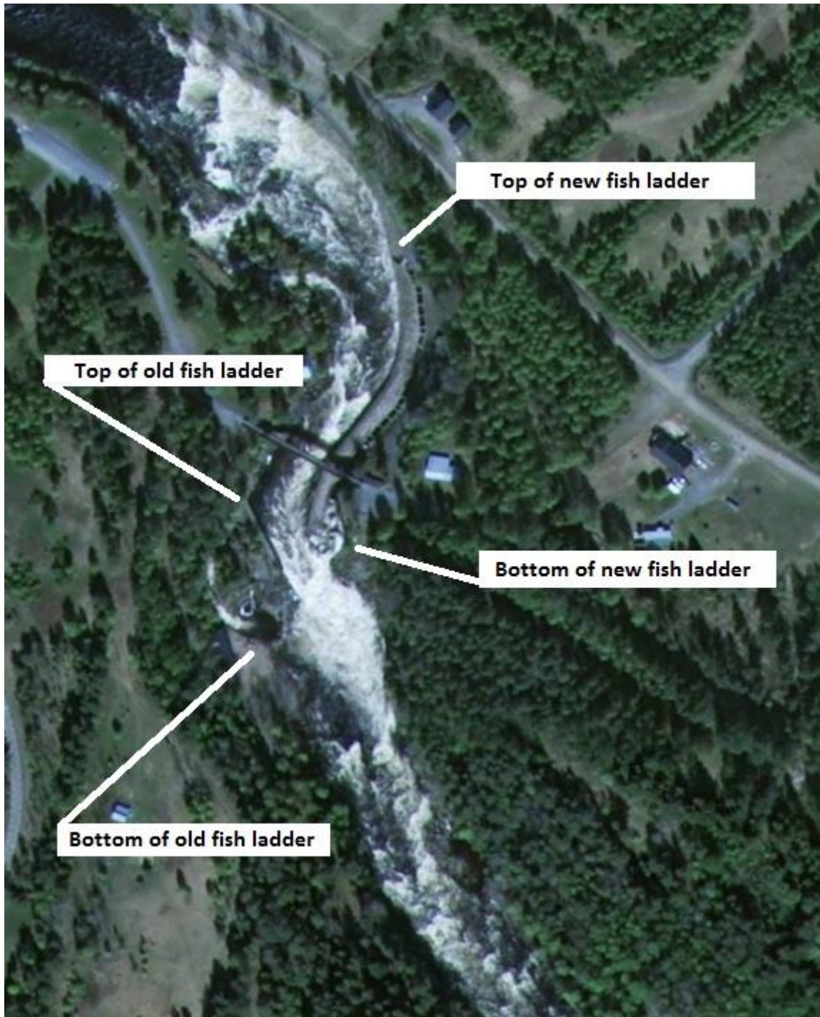
Figure 5: The two fish ladders at Fällfors in river Byskeälven 38 kilometres from the coast. The old fish ladder (on the left in the figure) is the fish ladder that salmon uses for upstream migration and also where the VAKI fish counter is situated. The new fish ladder (to the right in the figure) is rarely used by salmon. Fish can also pass this section without usage of the fish ladders. © Lantmäteriet, i2014/764.
