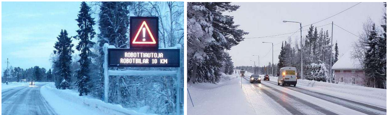
Figure 1 (a) VMS (left) and (b) safety car (right) warning drivers of automated vehicles' field-testing in the test section. (Pictures: (a) left Risto Kulmala and (b) right Sensible 4)
