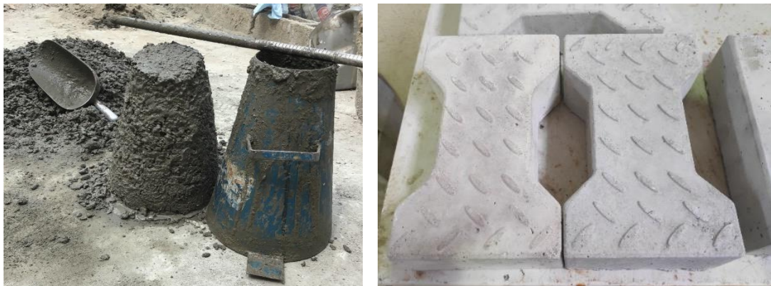
Figure 5. Slump of concrete mix ( left ); Interlocking concrete paver block ( right )
