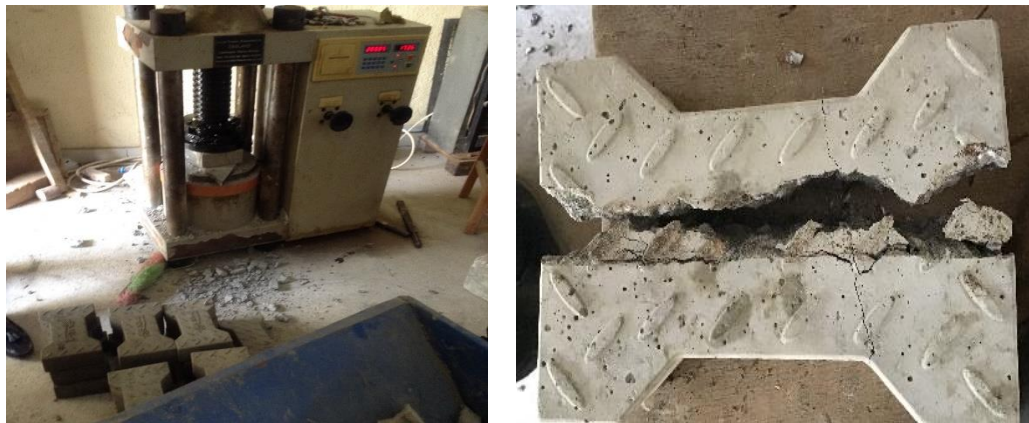
Figure 6. Testing of interlocking concrete paver ( left ); Failure mode of the paver sample containing WSF ( right )
