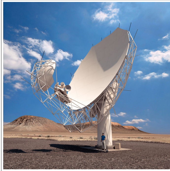
FIGURE 3.2: An artist's impression of a MeerKAT antenna to show the FI placed on the frame between the reflector and the sub-reflector. On the FI are also placed some feeds. Credit by the SKA Africa .
