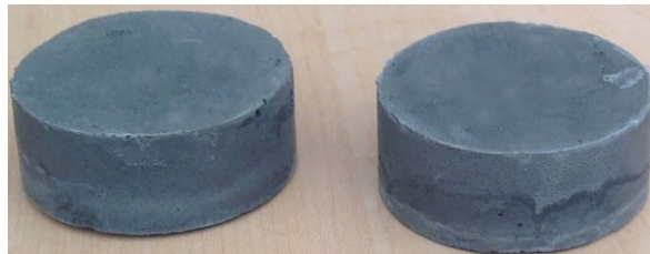
Figure 3. 36 – Specimens of cementitious mortar for thermal conductivity tests
