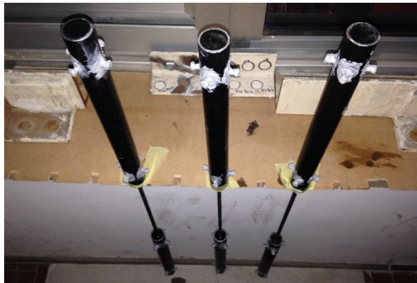
Figure 3. 51 - Specimens' preparation: CFRP bars embedded in gripping steel tubes
