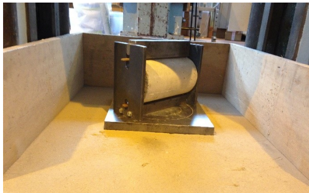
Figure 3. 40 - Apparatus for splitting cylinder test
