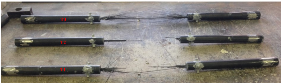
Figure 3. 55 - Failure mode of the tested specimens
