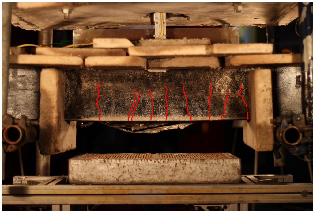
Figure 5. 60 –LochH-SL-2 after 90 min of heating
