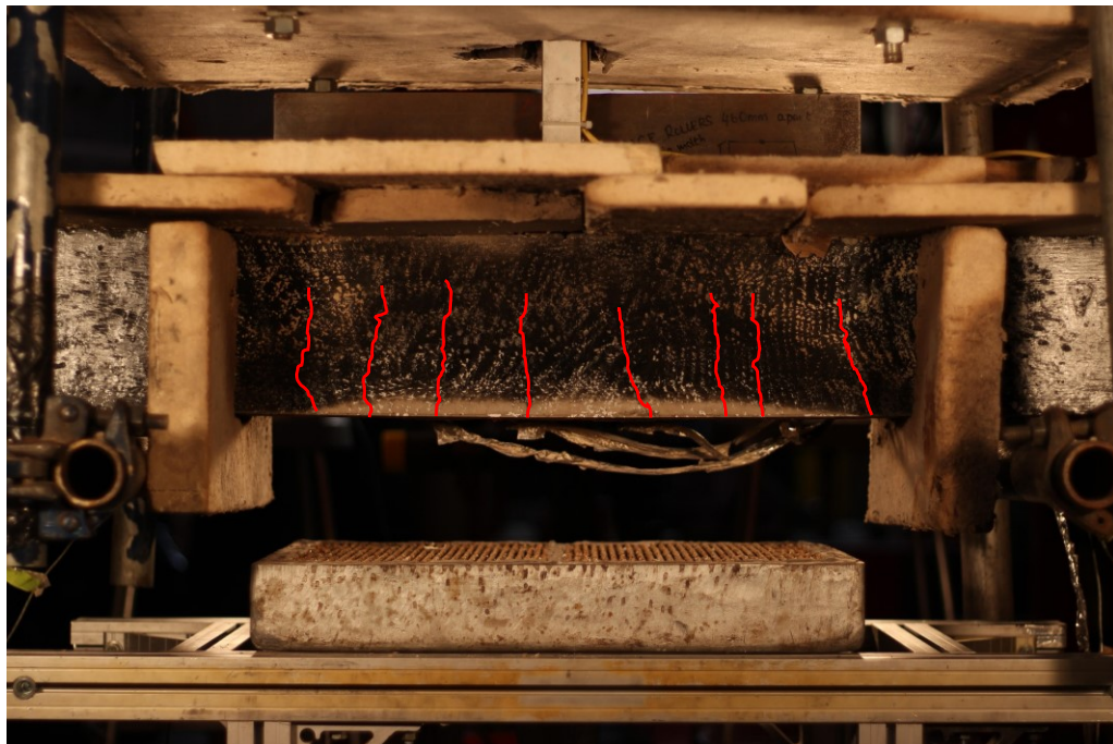
Figure 5. 59 –LochH-SL-1 after 90 min of heating
