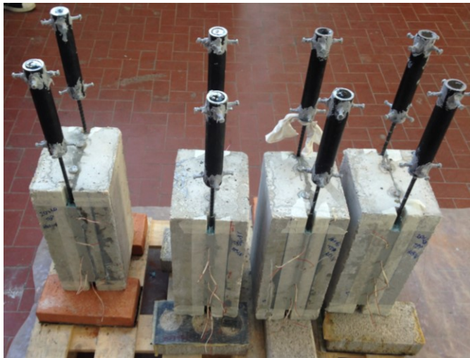
Figure 4. 10 – Installation of steel pipes at the end of the CFRP bars
