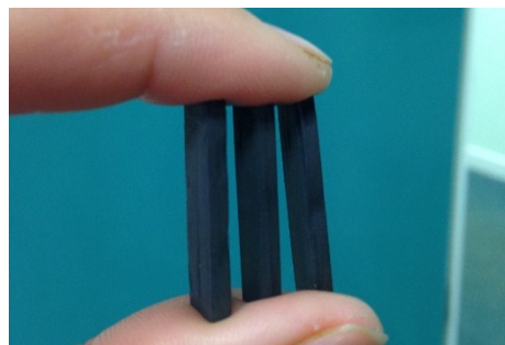
Figure 3. 4 - Specimens for DMA tests in single cantilever configuration
