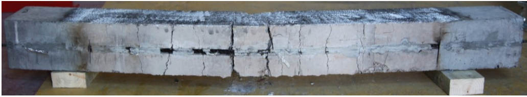
Figure 5. 66 – GloH-SL-1_residual after the residual test: a) Front side; b) Bottom side
