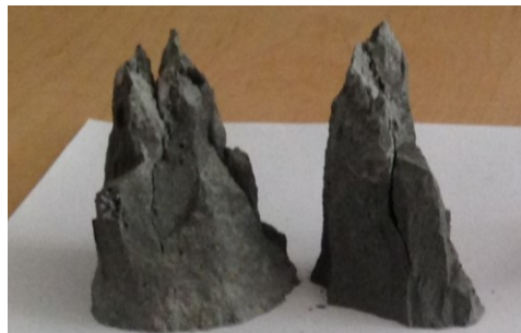
Figure 3. 50 - 810 Failure mode of the tested specimen
