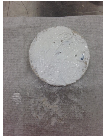
Figure 3. 33 - Specimen covered by the heat sink compound
