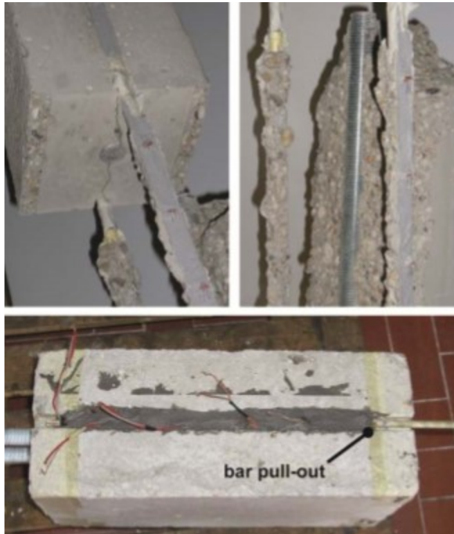
Figure 2. 13 – Splitting-related (top) and pull-out (bottom) failures in NSM specimens (Robin Round Tests – Bilotta et al, 2015)
