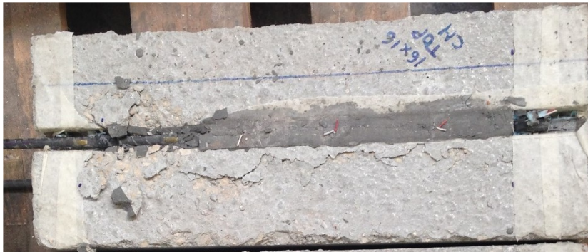
Figure 4. 15 – Failure at A/C interface after the main failure at B/A interface
