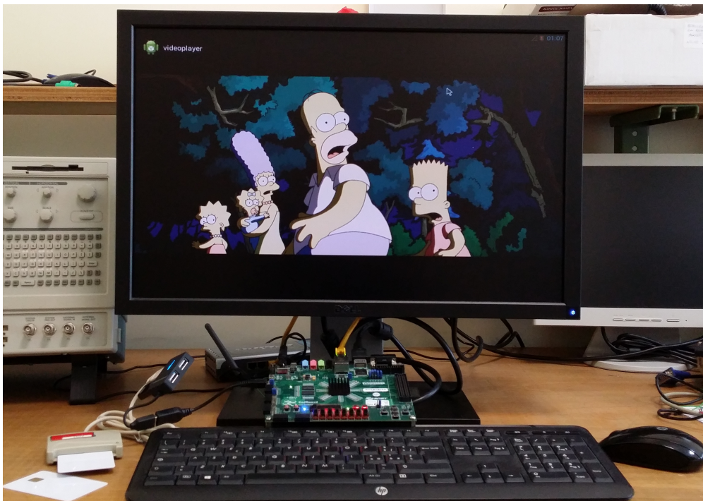
FIGURE 3.7: In the photo the Zedboard is running the Zedroid software stack on which it is downloaded an Android video player app with a hardware accelerator for the H.264 infra-frame prediction.
