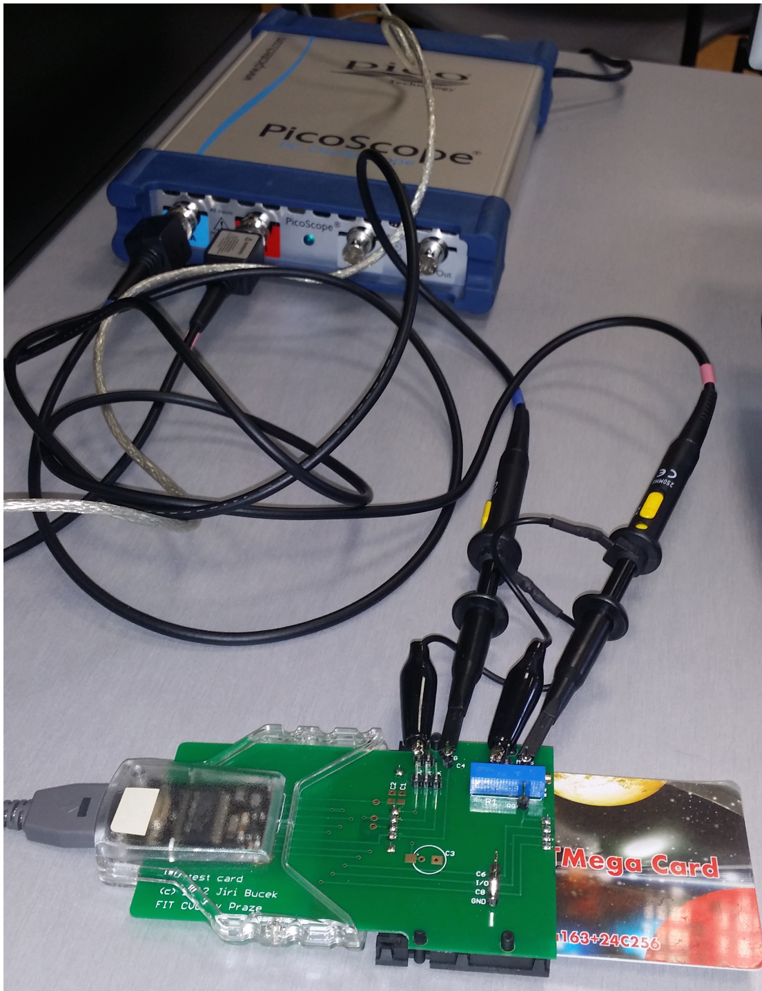
FIGURE 2.3: A side channel attack equipment to perform a power analysis on a smart card and extract the secret key. The attack was performed during the SCA session of TRUDEVICE summer school (Lisboa, July 2014).
