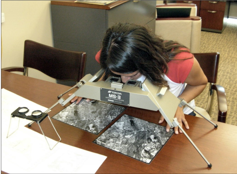
Figure 3.1 – A stereoscope used to analyze pairs of aerial photographs
