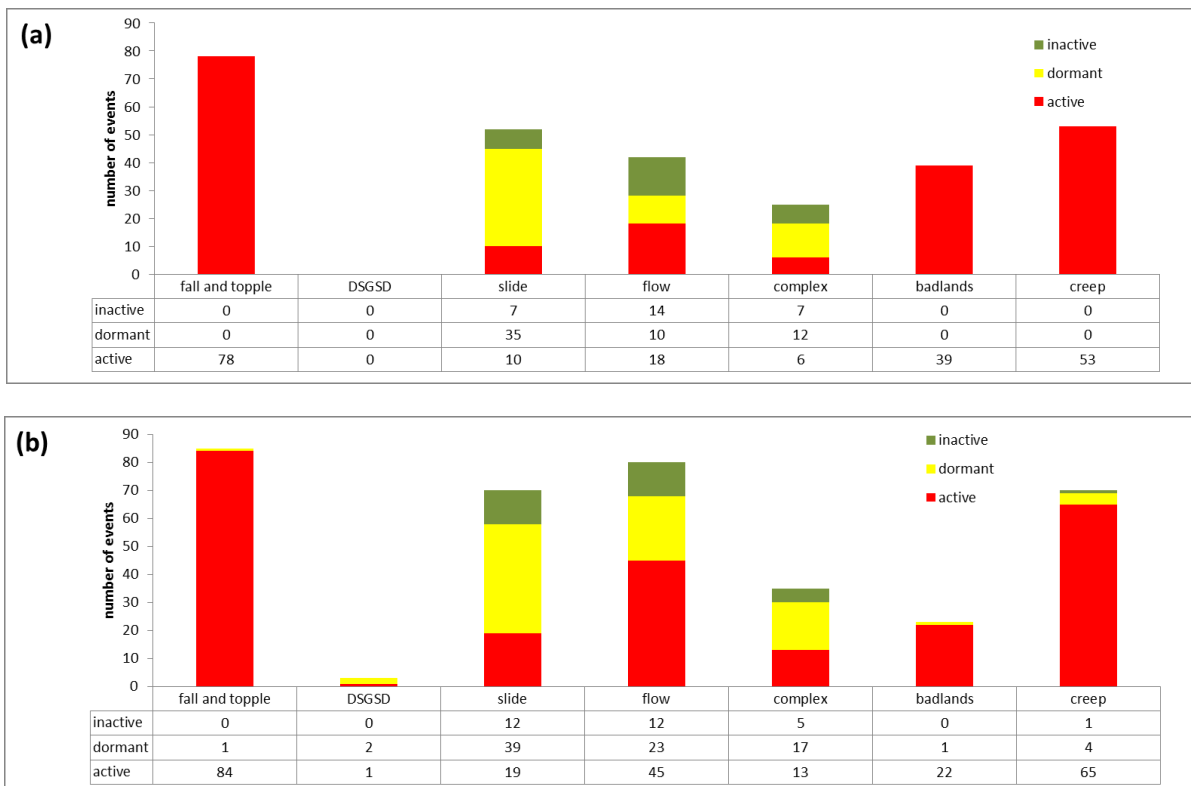
Figure 4.62 - Bar graphs showing the official (a) and new (b) Inventory Maps events according to landslide typology and state of activity.
