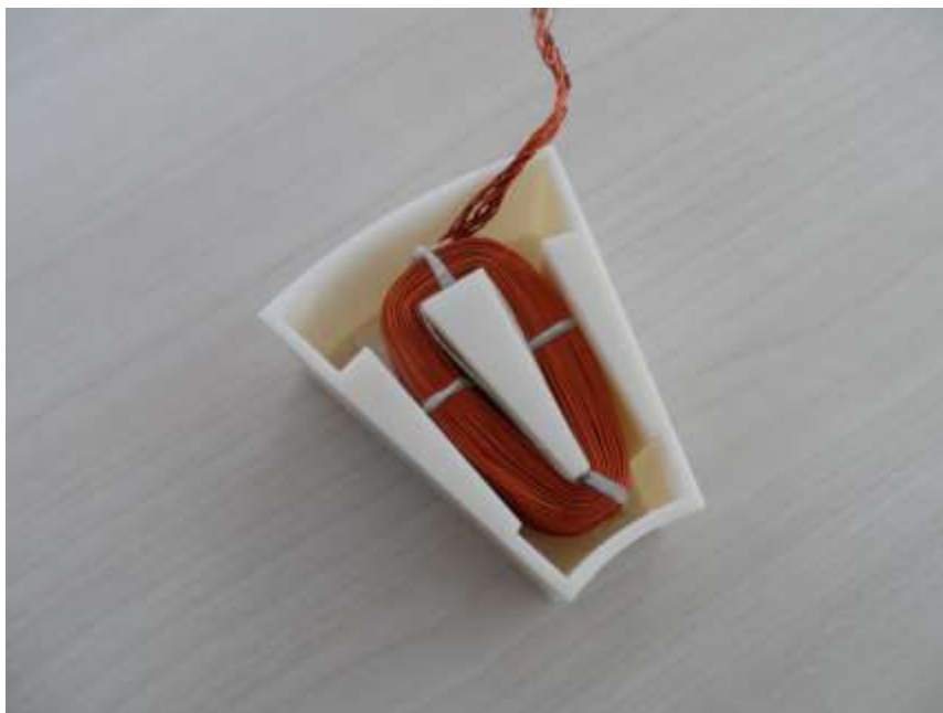
Fig.17.4 In the figure is shown a single coil which is wrapped around the teeth of machine. By courtesy of Umbra Cuscinetti SpA
