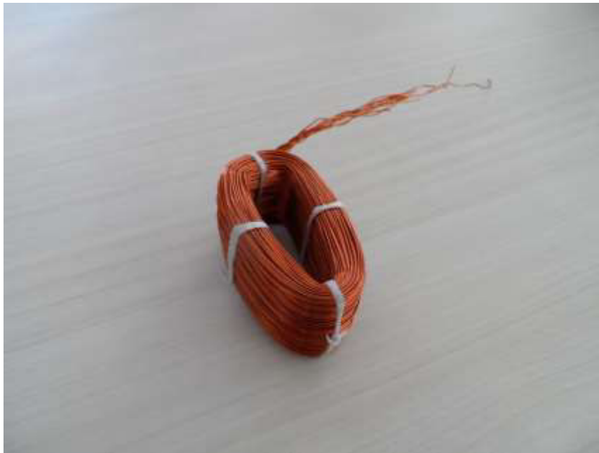
Fig.16.4 Single coil of windings (each phase is constituted by four type of this coil). By courtesy of Umbra Cuscinetti SpA
