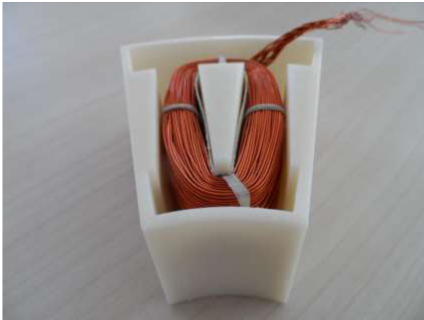
Fig.18.4 Frontal view of a single coil wrapped around the teeth of machine. By courtesy of Umbra Cuscinetti SpA
