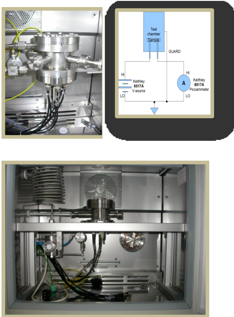
Fig. B1: Pictures of Gas Sensor Characterization System and corresponding circuitual scheme.
