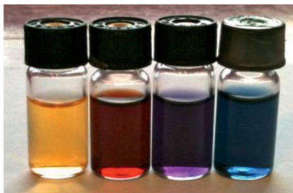
Figure 39. BBTZ as a four-state chromic system. From left to right: Z form; E form, protonated form, diprotonated form.
