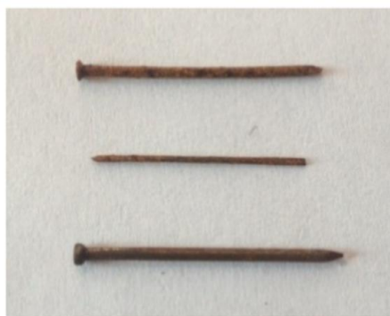
Figure 57. Rusty iron nails before (bottom) and after (middle) immersion in 36% HCl overnight and in the presence of 6 mM 1 (top)
