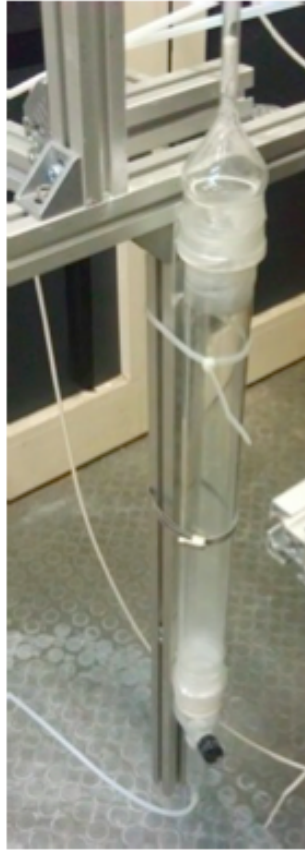
Fig. 4.51 Fluidized bed for seeding particles generation.
