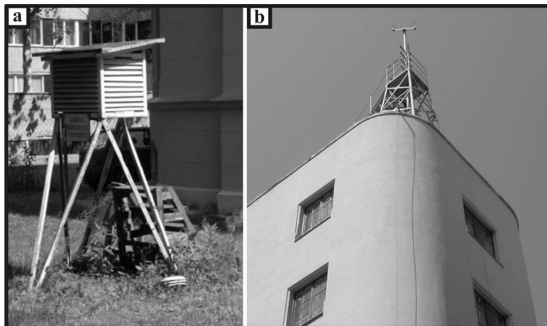
Fig. 4 Parts of the automatic station: the Stevenson screen (a) at the street level and (b) on the roof of the university building
