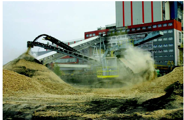
Figure 8. Production of the coal and biomass mixture for the cogeneration process
