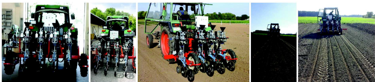
Figure 3. Testing of the precision plot seeder for medicinal and aromatic plants of the LfL with electrically driven seeding units and passive compensation of the slope inclination
