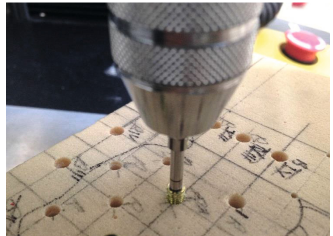
Fig. 2 Insertion of an implant in artificial bone block
