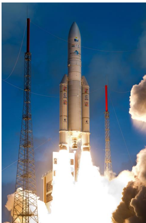
Figure 5. Lift-off picture of the Ariane 5 utilizing AP-based booster rockets. [37]
