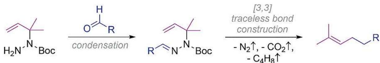
Figure 11 Graphical abstract of the article showing the condensation of the N -Boc- N -allylhydrazine with an aldehyde leading to a N -Boc- N -allylhydrazone. After [3,3]-sigmatropic rearrangement the desired isoprenylated product is formed
