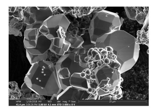
Figure S6. SEM image of  $Li_{38.7}Ce_{3.3}Ca_{5.7}[Li_2Si_{30}N_{59}]O_2F$  crystals.
