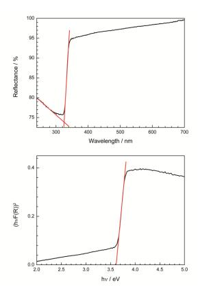
**Figure S3.** Top: Reflectance spectrum of undoped  $BaLi_2[Be_4O_6]$ . Bottom: Tauc plot (n = 1/2) for  $BaLi_2[Be_4O_6]$ . The band gap is estimated with both methods and is found in a range from 3.6–3.8 eV.
