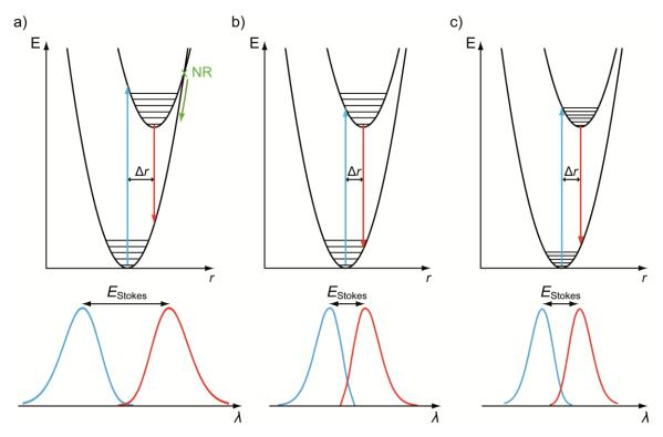
**Figure 3.** Configurational coordinate diagrams (top) and corresponding excitation and emission spectra (bottom), excitation blue and emission red, respectively.  $\Delta r$  gives the parabola offset between the ground states and the excited states. (a) Large *S* and  $\omega$ . NR indicates nonradiative decay from the excited state to the ground state. (b) Reduced *S*. (c) Reduced  $\omega$ .<sup>[17–19]</sup>
