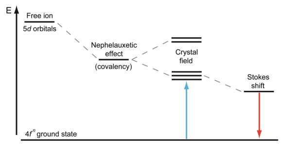
**Figure 2.** Stylized energy diagram showing major impacts on the excitation (blue arrow) and emission (red arrow) energy of  $Eu^{2+}$  and  $Ce^{3+.[15]}$
