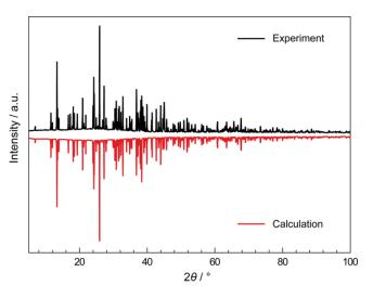
Figure 1. Measured X-ray powder diffraction pattern (black) and calculated pattern (red) for  $Li_{38.7}Y_{3.3}Ca_{5.7}[Li_2Si_{30}N_{59}]O_2F$ .
