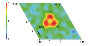
**Figure 4.** Residual electron density ( $F_{obs} - F_{calc}$ ) around special position 0,0,3/4 plotted with VESTA (scale bar in e<sup>-</sup> per a<sub>0</sub><sup>3</sup> with a<sub>0</sub> = Bohr radius).<sup>[44]</sup>
