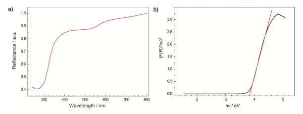
**Figure 5.** (a) Diffuse reflectance UV/Vis spectrum of  $Y_{23}Sr_{17}[Si_{38}O_{18}N_{67}]O_9$  after washing and annealing. (b) Tauc plot (black, n = 1/2) with tangent (red) at the inflection point.
