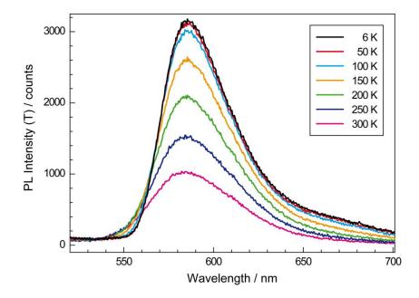
**Figure S6.** Temperature dependent emission spectra of  $La_{3-x}Ca_{1.5x}Si_6N_{11}$ :  $Eu^{2+}$  ( $x \approx 0.77$ ) with a nominal dopant concentration of 1 mol%.
