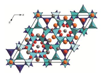
**Figure 2.** Crystal structure of  $Y_{23}Sr_{17}[Si_{38}O_{18}N_{67}]O_9$  along [001] with upper  $[Si_{38}O_{18}N_{67}]^{85-}$  layer turquoise, lower layer blue. Y and the Y/Sr site gray, Sr atoms orange, O atoms red, and N atoms blue; unit cell outlined in black.
