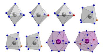
**Figure 3.** Coordination spheres of Lu and Ba sites in  $Lu_4Ba_2[Si_{12}O_2N_{16}C_3]:Eu^{2+}$  with O atoms red, O/N atoms blue, and N atoms orange.
