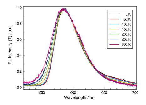
**Figure S7.** Normalized temperature dependent emission spectra of  $La_{3-x}Ca_{1.5x}Si_6N_{11}$ :  $Eu^{2+}$  (*x*  $\approx$  0.77) with a nominal dopant concentration of 1 mol%.
