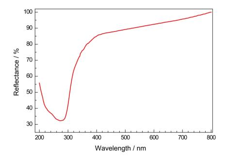
**Figure S5.** Diffuse reflectance UV/Vis spectrum of a nondoped  $La_{3-x}Ca_{1.5x}Si_6N_{11}$  ( $x \approx 0.77$ ) powder sample.
