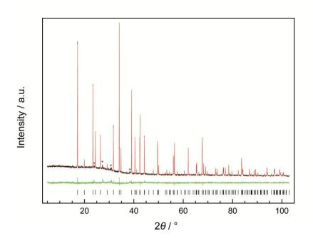
**Figure S2.** Crystal structure characterization of ultra-narrow band blue emitting  $AELi_2[Be_4O_6]:Eu^{2+}$  (AE = Sr, Ba). X-ray powder diffractogram (Cu K $\alpha_1$  radiation) of BLBO with the measured data (black line), calculated pattern based on Rietveld refinement data (red line), difference curve (green line), and tick marks (black) that give positions of Bragg reflections of BLBO; unknown side-phases are marked with asterisks.
