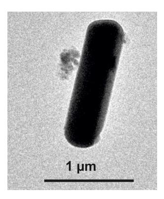
**Figure S2.** TEM image of the  $Lu_4Ba_2[Si_{12}O_2N_{16}C_3]$  crystallite used for the collection of single-crystal X-ray diffraction data.
