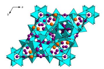
**Figure 2.** Crystal structure of  $Li_{38.7}RE_{3.3}Ca_{5.7}[Li_2Si_{30}N_{59}]O_2F$  (*RE* = Y, La, Ce), viewed along [001] with SiN<sub>4</sub> tetrahedra (turquoise), LiN<sub>4</sub> tetrahedra (violet), O/F atoms (red), Li atoms (violet), and *RE*/Ca atoms (orange). Unit cell in black.
