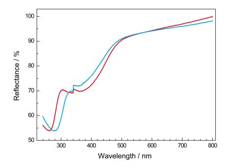
**Figure S8.** Diffuse reflectance UV/Vis spectra of doped samples of  $Lu_4Ba_2[Si_{12}O_2N_{16}C_3]:Eu^{2+}$  (red) and  $Y_4Ba_2[Si_{12}O_2N_{16}C_3]:Eu^{2+}$  (blue). The artifacts around 340 nm correspond to the lamp-switch.
