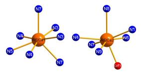
Figure 4. Coordination spheres of *RE*/Ca sites in  $Li_{38.7}RE_{3.3}Ca_{5.7}[Li_2Si_{30}N_{59}]O_2F$  (*RE* = La, Ce, Y).
