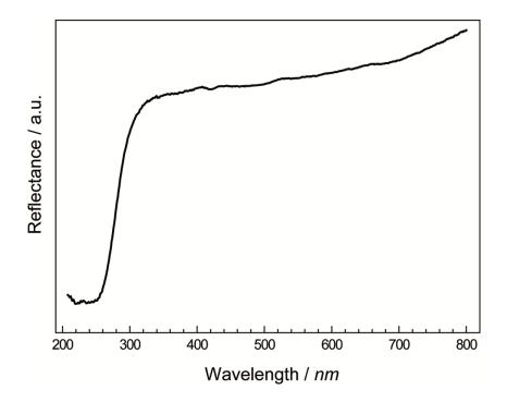
Figure S4. UV/Vis spectrum of nondoped Y<sub>4</sub>Ba<sub>2</sub>[Si<sub>9</sub>ON<sub>16</sub>]O.
