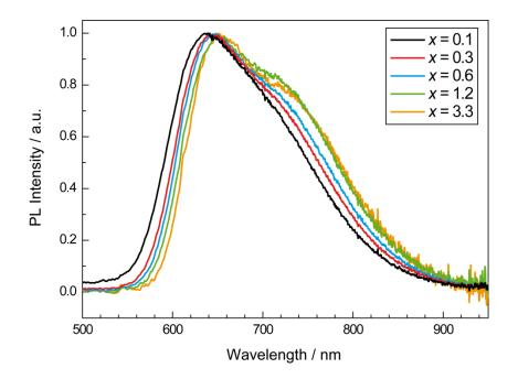
Figure S12. Emission spectra of  $Li_{38.7}La_{3.3-x}Ce_xCa_{5.7}[Li_2Si_{30}N_{59}]O_2F$  (x = 0.1–3.3).
