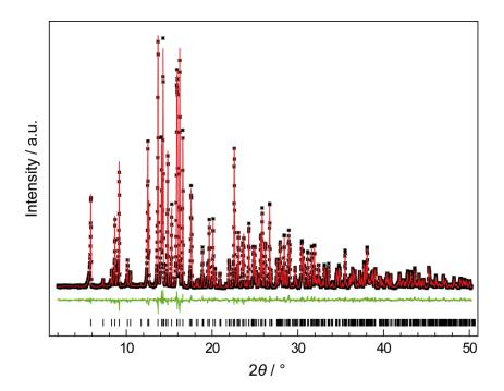
**Figure S1.** Rietveld refinement based on the XRD pattern of  $Ba_2Si_5N_8$  which was used as starting material (Mo K $\alpha_1$ ,  $\lambda = 0.7093$  Å).<sup>[1]</sup> Measured histogram (black stars), Rietveld fit (red line), difference plot (green line). Only lattice parameters and profile functions were refined.
