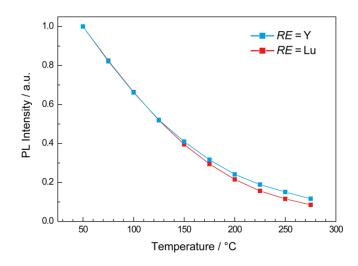
**Figure 6.** Thermal quenching data for  $RE_4Ba_2[Si_{12}O_2N_{16}C_3]:Eu^{2+}$  (RE = Lu, Y).
