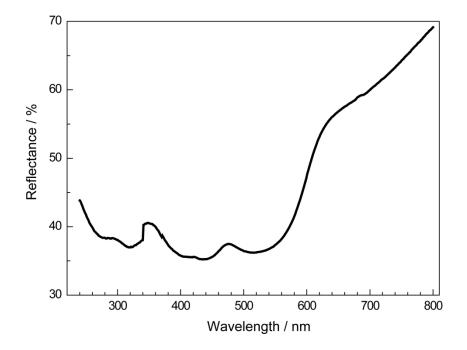
**Figure S11.** Diffuse reflectance UV/Vis spectrum of a  $Li_{38.7}Ce_{3.3}Ca_{5.7}[Li_2Si_{30}N_{59}]O_2F$  powder sample. The compound shows strong absorption in the visible to blue range with absorption bands around 530 nm and 420 nm. The artifact around 340 nm corresponds to the lamp switch.
