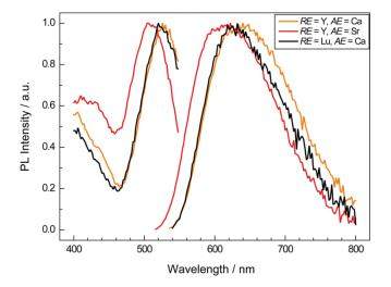
**Figure 1.** Normalized excitation and emission spectra of particles with the nominal composition  $Li_{38.7}Y_{3.3}Sr_{5.7}[Li_2Si_{30}N_{59}]O_2F:Ce^{3+}$  and  $Li_{38.7}Lu_{3.3}Ca_{5.7}[Li_2Si_{30}N_{59}]O_2F:Ce^{3+}$  compared to spectra of  $Li_{38.7}Y_{3.3}Ca_{5.7}[Li_2Si_{30}N_{59}]O_2F:Ce^{3+}$ .
