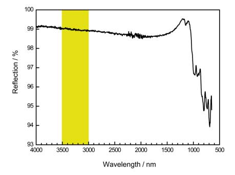
**Figure S3.** ATR-FTIR spectrum of a  $La_{3-x}Ca_{1.5x}Si_6N_{11}$ :  $Eu^{2+}$  ( $x \approx 0.77$ ) powder sample. Typical region for N–H vibrations colored yellow.
