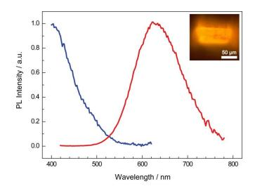
Figure 7. Excitation (blue) and emission spectra (red) for crystals of Y<sub>26</sub>Ba<sub>6</sub>[Si<sub>22</sub>O<sub>19</sub>N<sub>36</sub>]O<sub>16</sub>:Eu<sup>2+</sup>.
