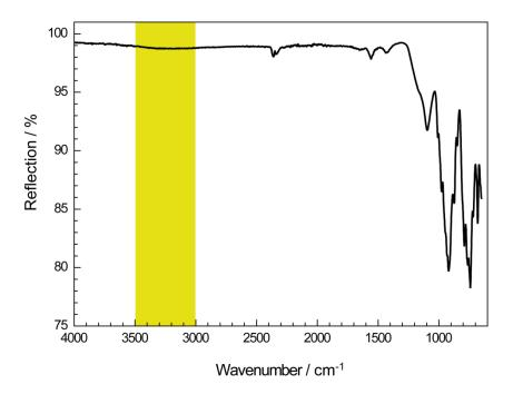
**Figure S1.** ATR-FTIR spectrum of a Y<sub>4</sub>Ba<sub>2</sub>[Si<sub>9</sub>ON<sub>16</sub>]O powder sample. Typical region for N–H and O–H vibrations colored yellow.
