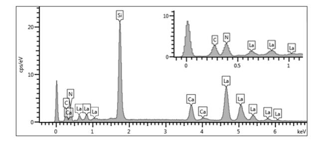
**Figure S2.** Exemplary EDX spectrum measured on a  $La_{3-x}Ca_{1.5x}Si_6N_{11}$ :  $Eu^{2+}$  ( $x \approx 0.77$ ) crystal. The carbon peak originates from the carbon coating as well as the carbon pad on which the crystals were mounted. The magnified region from 0–1 keV illustrates that no significant amounts of O (0.525 keV) and no F (0.677 keV) were detected.
