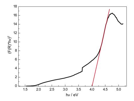
Figure S10. Tauc plot (n = 1/2) for the nondoped Li<sub>38.7</sub>Y<sub>3.3</sub>Ca<sub>5.7</sub>[Li<sub>2</sub>Si<sub>30</sub>N<sub>59</sub>]O<sub>2</sub>F powder sample.
