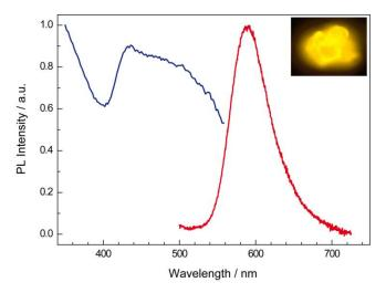
**Figure 5.** Excitation (blue) and emission (red,  $\lambda_{exc} = 440 \text{ nm}$ ) spectra of  $La_{3-x}Ca_{1.5x}Si_6N_{11}:Eu^{2+1}$  ( $x \approx 0.77$ ) bulk material with a nominal dopant concentration of 1%.
