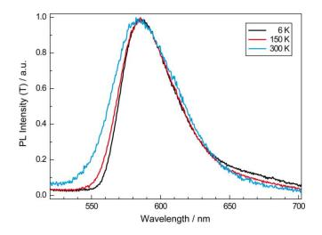
**Figure 8.** Normalized temperature dependent emission spectra for  $La_{3-x}Ca_{1.5x}Si_6N_{11}$ :  $Eu^{2+}$  ( $x \approx 0.77$ ) with 1 mol% Eu (nominal).
