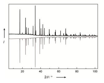
**Figure 2.** Crystal structure characterization of ultra-narrow band blue emitting  $AELi_2[Be_4O_6]:Eu^{2+}$  (AE = Sr, Ba). X-ray powder pattern of BLBO with the measured data (black line) and calculated pattern based on Rietveld refinement data (gray line).
