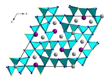
**Figure 1.** Crystal structure of  $RE_4Ba_2[Si_{12}O_2N_{16}C_3]:Eu^{2+}$  (RE = Lu, Y), viewed along [001]. SiC(O/N)<sub>3</sub> tetrahedra turquoise; *RE* atoms gray; Ba atoms violet; O atoms red; O/N atoms blue; N atoms orange, C atoms yellow.
