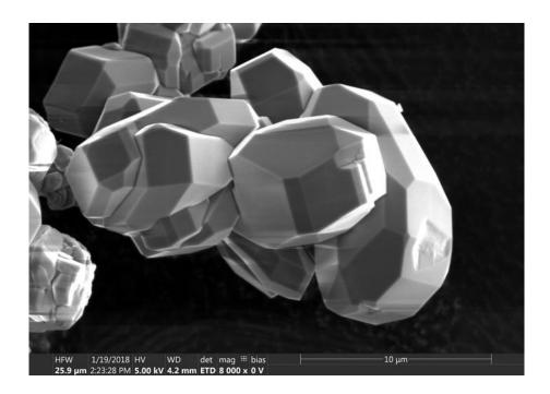
Figure S5. SEM image of  $Li_{38.7}La_{3.3}Ca_{5.7}[Li_2Si_{30}N_{59}]O_2F$  crystals.
