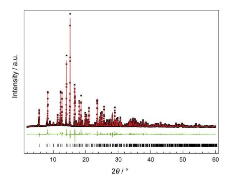
**Figure S4.** Rietveld refinement of data collected from a  $La_{3-x}Ca_{1.5x}Si_6N_{11}$ :  $Eu^{2+}$  ( $x \approx 0.77$ ) sample. Experimental PXRD data as black stars, Rietveld fit red, difference plot green, reflection positions of  $La_{3-x}Ca_{1.5x}Si_6N_{11}$ :  $Eu^{2+}$  ( $x \approx 0.77$ ) as black bars.
