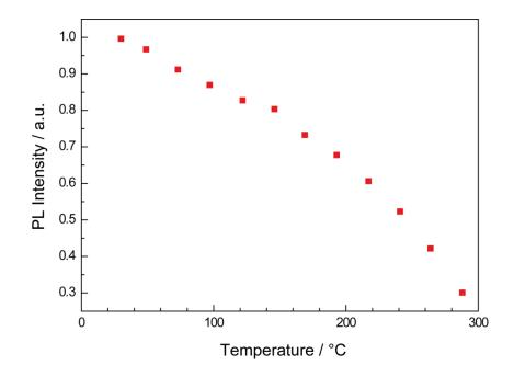
Figure S6. Thermal quenching data for  $Y_4Ba_2[Si_9ON_{16}]O:Eu^{2+}$ .
