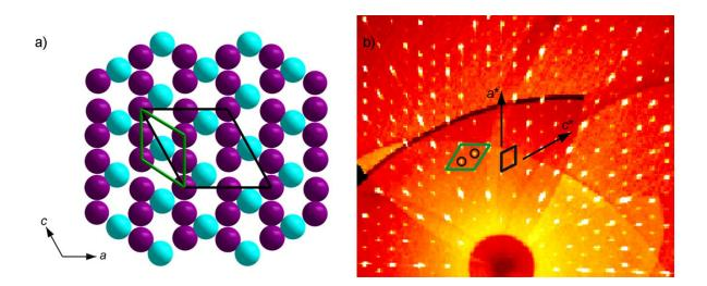
**Figure 4.** (a) Layer of Ba atoms forming Kagomé nets in the *ac*-plane. Ba atoms located in silicate cages, turquoise; Ba atoms outside cages, violet. Small pseudohexagonal unit cell, green; actual unit cell including the superstructure, black. Radius of Ba atoms  $\approx 2.4$  Å. (b) *h*0*l* reciprocal lattice section with corresponding green and black reciprocal cells. Superstructure reflections marked by black circles only described by black reciprocal cell.
