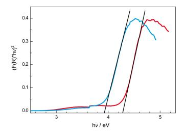
**Figure 4.** Tauc plots (n = 1/2) for  $RE_4Ba_2[Si_{12}O_2N_{16}C_3]:Eu^{2+}$ ; plot for RE = Lu red, plot for RE = Y blue, tangents at the inflection points black.
