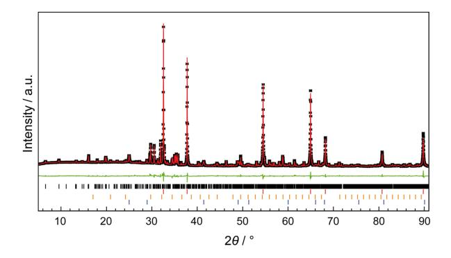
**Figure S3.** Rietveld refinement of data collected from a  $Lu_4Ba_2[Si_9ON_{16}]O:Eu^{2+}$  sample. Reflection positions for  $Lu_4Ba_2[Si_9ON_{16}]O:Eu^{2+}$  black (43 wt%), LuN red (43 wt%),  $Lu_2O_3$  orange (6 wt%),  $BaF_2$  blue bars (8 wt%), respectively.
