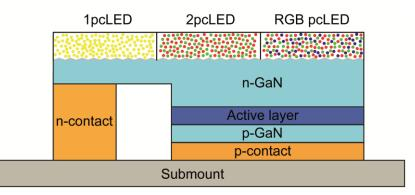
**Figure 1.** Schematic build-up of a pcLED. A thin-film, flip-chip LED emitting in the blue or near-UV excites yellow (1pcLED), red and green (2pcLED), or red, green and blue phosphors (RGB). Additive color-mixing results in the emission of white light.<sup>[7]</sup>
