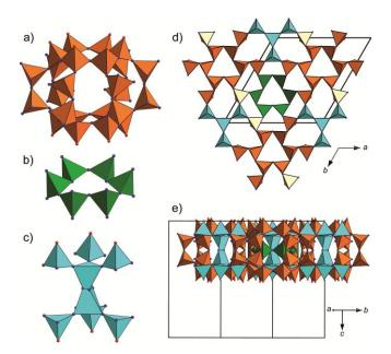
**Figure 3.** (a) Cage. (b) *Sechser* ring. (c) Entity of eight tetrahedra. (d)  $[Si_{38}O_{18}N_{67}]^{85-}$  layer along [001]. (e)  $[Si_{38}O_{18}N_{67}]^{85-}$  layer along [210]; unit cells outlined in black.
