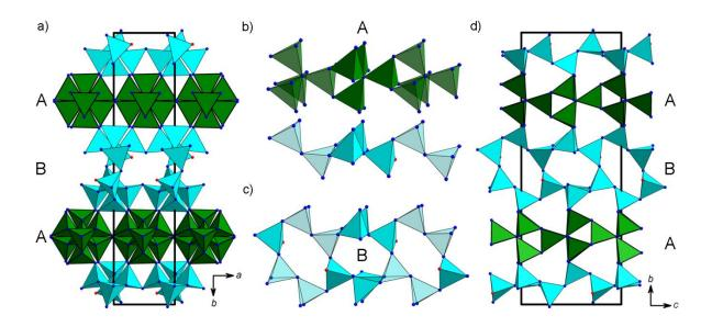
**Figure 3.** (a) Three-dimensional silicate network of  $RE_4Ba_2[Si_9ON_{16}]O:Eu^{2+}$  (RE = Y, Lu) along [001] with highly condensed strands of star-shaped  $[N^{[4]}(SiN_3)_4]$  units (A, green) and less condensed strands (B, turquoise). (b) A strands of  $[N^{[4]}(SiN_3)_4]$  units (green) and half a B strand (turquoise). (c) B strand. (d) Structure in projection along [100]. N atoms blue, O atoms red, and unit cell outlined in black.
