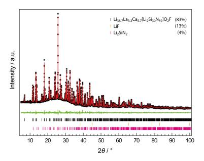
**Figure S2.** Rietveld refinement of data collected from a  $Li_{38.7}La_{3.3}Ca_{5.7}[Li_2Si_{30}N_{59}]O_2F$  sample ( $\lambda = 1.54056$  Å). Experimental PXRD data as black stars, Rietveld fit red, difference plot green. Reflection positions of  $Li_{38.7}La_{3.3}Ca_{5.7}[Li_2Si_{30}N_{59}]O_2F$  as black bars. The sample contains LiF formed during the metathesis reaction (orange bars, 13 wt%), and small amounts of  $Li_2SiN_2$  (magenta bars, 4 wt%).
