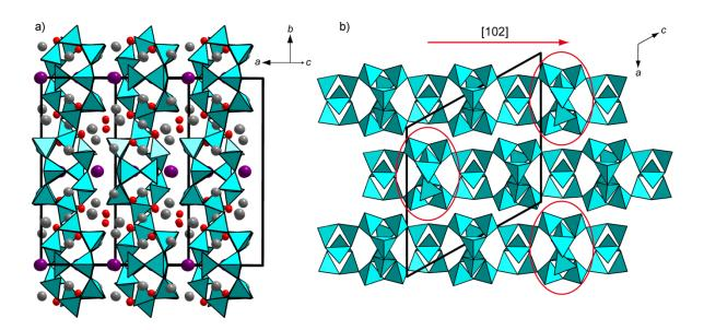
**Figure 2.** (a) Crystal structure of  $RE_{26}Ba_6[Si_{22}O_{19}N_{36}]O_{16}$ :Eu<sup>2+</sup> (RE = Y, Tb), viewing direction [102]. (b)  $[Si_{22}O_{19}N_{36}]^{58-}$  layers, viewed along [010] with shift along [102] indicated by red arrow. SiN<sub>4</sub>/Si(O/N)<sub>4</sub> tetrahedra, turquoise; Y/Tb atoms, gray; Ba atoms, violet; and noncondensed O atoms, red.
