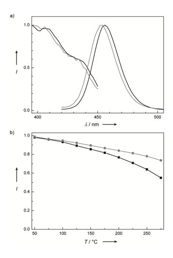
**Figure 1.** Photoluminescence properties of ultra-narrow band blue emitting  $AELi_2[Be_4O_6]:Eu^{2+}$ (AE = Sr, Ba). (a) Excitation and emission spectra of  $BaLi_2[Be_4O_6]:Eu^{2+}$  (gray) and  $SrLi_2[Be_4O_6]:Eu^{2+}$  (black) for  $\lambda_{exc} = 400$  nm. (b) Temperature dependence of the relative integrated photoluminescence intensity for BLBO (gray) and SLBO (black), revealing a decrease at 200 °C of only 17 and 24%, respectively, compared to room-temperature QE.
