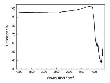
**Figure S5.** ATR-FTIR spectrum of a  $Lu_4Ba_2[Si_{12}O_2N_{16}C_3]:Eu^{2+}$  powder sample. Bands at 2345 cm<sup>-1</sup> belong to the asymmetric stretching vibration of CO<sub>2</sub>. No O–H and N–H bands are observed in the typical region.
