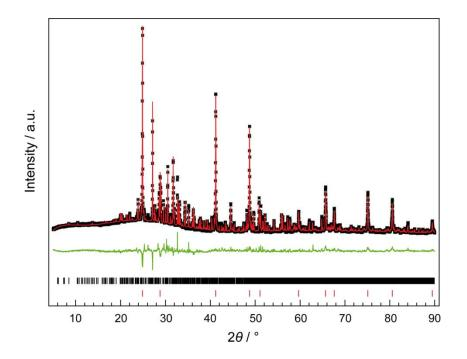
**Figure S2.** Rietveld refinement of data collected for an unwashed  $Y_{26}Ba_6[Si_{22}O_{19}N_{36}]O_{16}$ :Eu<sup>2+</sup> sample. Experimental data as black stars, Rietveld fit as red line and difference plot as green line. Reflection positions for  $Y_{26}Ba_6[Si_{22}O_{19}N_{36}]O_{16}$ :Eu<sup>2+</sup> (black bars, 70 wt%) and BaF<sub>2</sub> (red bars, 30 wt%).
