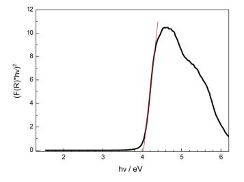
**Figure 4.** Tauc plot (n = 1/2) for nondoped La<sub>3-x</sub>Ca<sub>1.5x</sub>Si<sub>6</sub>N<sub>11</sub> ( $x \approx 0.77$ ).
