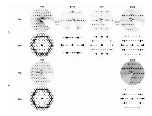
**Figure S7.** SAED patterns of  $Lu_4Ba_2[Si_{12}O_2N_{16}C_3]$  (top) and  $Y_4Ba_2[Si_{12}O_2N_{16}C_3]$  (bottom) with simulations and experimental tilt angles (blue) and theoretical tilt angles (red).
