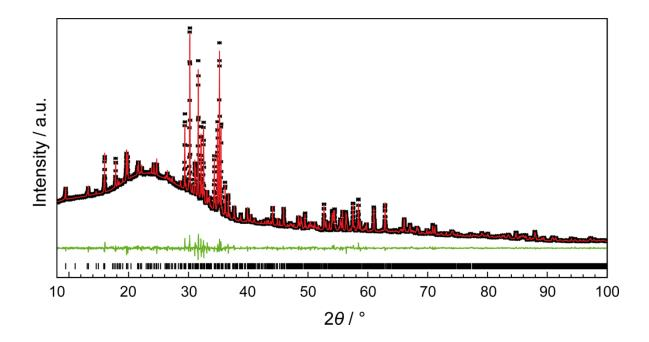
**Figure S2.** Rietveld refinement of data collected from a  $Y_4Ba_2[Si_9ON_{16}]O:Eu^{2+}$  sample. Reflection positions for  $Y_4Ba_2[Si_9ON_{16}]O:Eu^{2+}$  as black bars.
