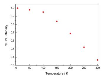
**Figure 7.** Relative integrated emission intensity of  $La_{3-x}Ca_{1.5x}Si_6N_{11}$ :  $Eu^{2+}$  ( $x \approx 0.77$ ) with 1 mol% Eu (nominal).
