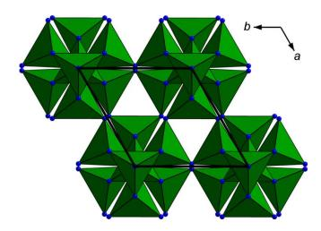
**Figure 4.** Silicate network of  $BaYb[Si_4N_7]$  along [001],  $SiN_4$  tetrahedra green, N atoms blue, and unit cell outlined in black.
