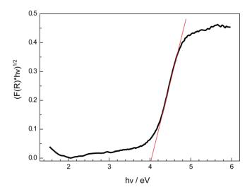
**Figure 6.** Tauc plot (n = 2) for nondoped Y<sub>4</sub>Ba<sub>2</sub>[Si<sub>9</sub>ON<sub>16</sub>]O.
