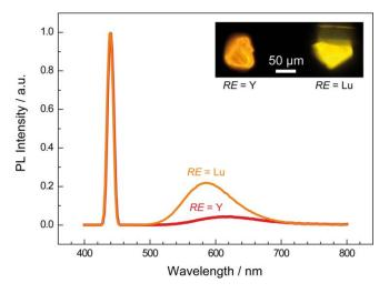
**Figure 9.** Comparison of luminescence intensities of  $Y_4Ba_2[Si_9ON_{16}]O:Eu^{2+}$  (red) and  $Lu_4Ba_2[Si_9ON_{16}]O:Eu^{2+}$  (orange) single crystals. Normalized excitation peaks at 440 nm.
