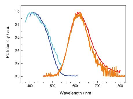
**Figure S5**.  $Y_4Ba_2[Si_9ON_{16}]O:Eu^{2+}$  single crystal: normalized excitation spectrum ( $\lambda_{mon} = 636$  nm) dark blue, normalized emission spectrum ( $\lambda_{exc} = 440$  nm) red;  $Y_4Ba_2[Si_9ON_{16}]O:Eu^{2+}$  powder: normalized excitation spectrum ( $\lambda_{mon} = 636$  nm) cyan, normalized emission spectrum ( $\lambda_{exc} = 440$  nm) orange.
