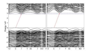
**Figure 7.** Calculated band structures for Y<sub>4</sub>Ba<sub>2</sub>[Si<sub>9</sub>ON<sub>16</sub>]O (left) and Lu<sub>4</sub>Ba<sub>2</sub>[Si<sub>9</sub>ON<sub>16</sub>]O (right). Red arrows indicate indirect transitions.
