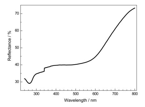
**Figure S9.** Diffuse reflectance UV/Vis spectrum of a nondoped  $Li_{38.7}Y_{3.3}Ca_{5.7}[Li_2Si_{30}N_{59}]O_2F$  powder sample. The artifact around 340 nm corresponds to the lamp switch.
