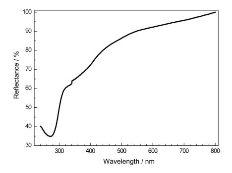
**Figure S8.** Diffuse reflectance UV/Vis spectrum of a nondoped  $Li_{38.7}La_{3.3}Ca_{5.7}[Li_2Si_{30}N_{59}]O_2F$  powder sample. The artifact around 340 nm corresponds to the lamp switch.
