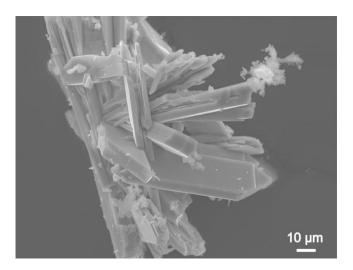
Figure 1. SEM image of Y<sub>4</sub>Ba<sub>2</sub>[Si<sub>9</sub>ON<sub>16</sub>]O:Eu<sup>2+</sup>.
