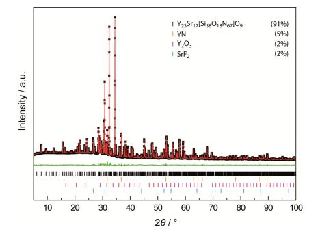
**Figure 1.** Rietveld refinement based on the XRD pattern of a washed and annealed  $Y_{23}Sr_{17}[Si_{38}O_{18}N_{67}]O_9$  sample with measured histogram (black stars), Rietveld fit (red line), difference plot (green line), and positions of reflections (bars):  $Y_{23}Sr_{17}[Si_{38}O_{18}N_{67}]O_9$  (black), YN (orange),  $Y_2O_3$  (magenta), SrF<sub>2</sub> (cyan); phase proportions in wt %.
