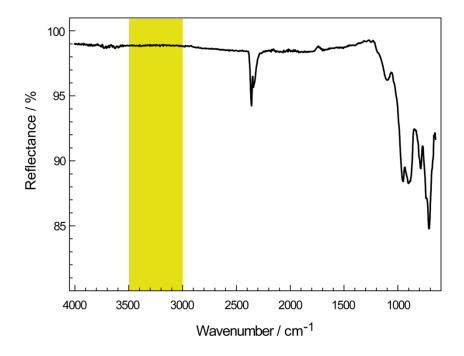
**Figure S1.** ATR-FTIR spectrum of a  $Y_{26}Ba_6[Si_{22}O_{19}N_{36}]O_{16}:Eu^{2+}$  powder sample. Typical region for N–H and O–H vibrations colored yellow. Bands at 2345 cm<sup>-1</sup> belong to the asymmetric stretch vibration of CO<sub>2</sub>.
