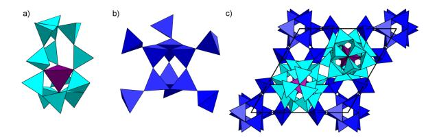
**Figure 3.** (a) Cage of SiN<sub>4</sub> tetrahedra (turquoise) containing a LiN<sub>4</sub> tetrahedra (violet). (b) Double dreier ring with additional SiN<sub>4</sub> tetrahedra at the vertices (blue). (c) Three-dimensional tetrahedra network, viewing direction [001].
