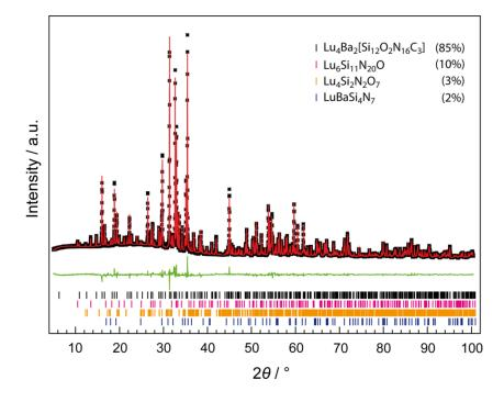
**Figure S3.** Rietveld refinement based on the XRD pattern (Cu K $\alpha_1$ ,  $\lambda = 1.54056$  Å) of a Lu<sub>4</sub>Ba<sub>2</sub>[Si<sub>12</sub>O<sub>2</sub>N<sub>16</sub>C<sub>3</sub>] sample with measured histogram (black stars), Rietveld fit (red line), difference plot (green line), and positions of reflections (bars).
