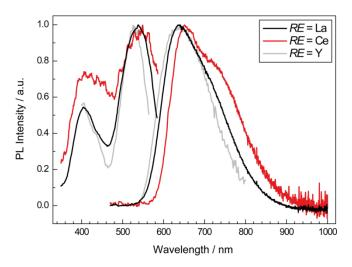
**Figure 6.** Normalized excitation and emission spectra ( $\lambda_{exc} = 440 \text{ nm}$ ) of Li<sub>38.7</sub>*RE*<sub>3.3</sub>Ca<sub>5.7</sub>[Li<sub>2</sub>Si<sub>30</sub>N<sub>59</sub>]O<sub>2</sub>F (*RE* = La, Ce, Y). Samples with *RE* = La, Y were doped with 3 atom% Ce (nominal).
