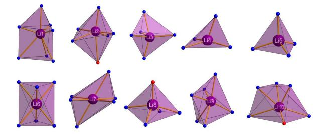
**Figure S7.** Coordination spheres of the Li sites in  $Li_{38.7}RE_{3.3}Ca_{5.7}[Li_2Si_{30}N_{59}]O_2F$  (*RE* = La, Ce, Y). Due to its regular tetrahedral coordination, Li5 is listed as cation with contribution to the network structure.
