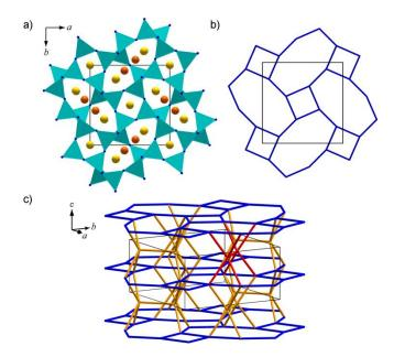
**Figure 2.** (a) Crystal structure of  $La_{3-x}Ca_{1.5x}Si_6N_{11}:Eu^{2+}$  in projection along [001] with SiN<sub>4</sub> tetrahedra (turquoise), N atoms (blue), La,Ca atoms (yellow), and Ca atoms (orange). (b) Topological representation of layers formed by *achter* and *vierer* rings (blue). (c) Topological representation with layer-linking pairs (yellow, one unit highlighted in red). Unit cell shown in black.
