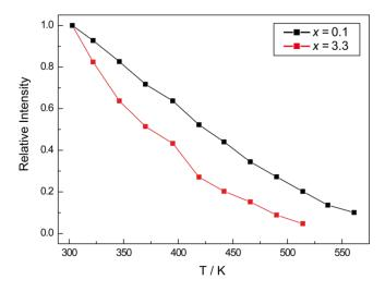
**Figure 7.** Temperature dependent integrated luminescence intensities of Li<sub>38.7</sub>La<sub>3.3-x</sub>Ce<sub>x</sub>Ca<sub>5.7</sub>[Li<sub>2</sub>Si<sub>30</sub>N<sub>59</sub>]O<sub>2</sub>F.
