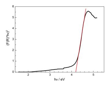
Figure 6. Tauc plot (n = 1/2) for  $Y_{26}Ba_6[Si_{22}O_{19}N_{36}]O_{16}:Eu^{2+}$ .
