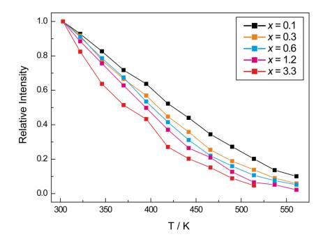
**Figure S13.** Temperature dependent integrated luminescence intensities of Li<sub>38.7</sub>La<sub>3.3-x</sub>Ce<sub>x</sub>Ca<sub>5.7</sub>[Li<sub>2</sub>Si<sub>30</sub>N<sub>59</sub>]O<sub>2</sub>F.
