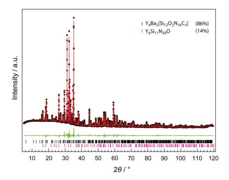
**Figure S4.** Rietveld refinement based on the XRD pattern (Cu K $\alpha_1$ ,  $\lambda = 1.54056$  Å) of a Y<sub>4</sub>Ba<sub>2</sub>[Si<sub>12</sub>O<sub>2</sub>N<sub>16</sub>C<sub>3</sub>] sample with measured histogram (black stars), Rietveld fit (red line), difference plot (green line), and positions of reflections (bars).
