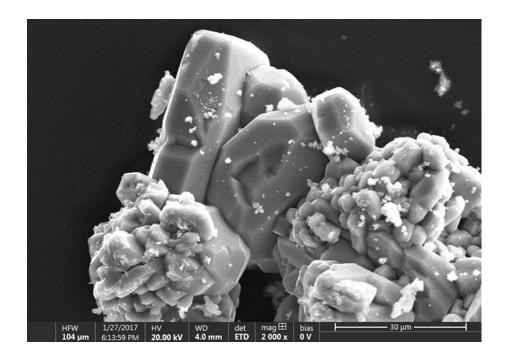
Figure S4. SEM image of  $Li_{38.7}Y_{3.3}Ca_{5.7}[Li_2Si_{30}N_{59}]O_2F$  crystals.
