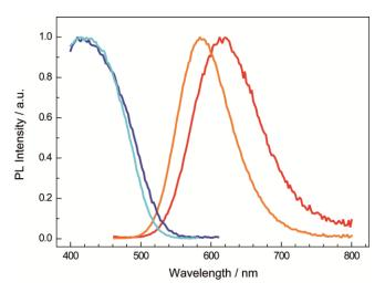
**Figure 8.**  $Y_4Ba_2[Si_9ON_{16}]O:Eu^{2+}$ : normalized excitation spectrum ( $\lambda_{mon} = 636$  nm) dark blue, normalized emission spectrum ( $\lambda_{exc} = 440$  nm) red;  $Lu_4Ba_2[Si_9ON_{16}]O:Eu^{2+}$ : normalized excitation spectrum ( $\lambda_{mon} = 600$  nm) cyan, emission spectrum ( $\lambda_{exc} = 440$  nm) orange.
