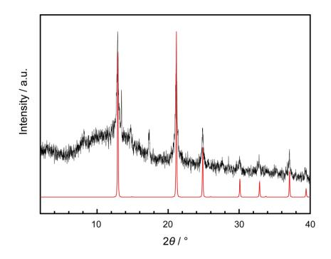
**Figure S1.** Experimental PXRD data (black, Mo K $\alpha_1$  radiation, Ge(111) monochromator, Mythen1K detector) of colorless powder deposited on the silica glass reactor wall during the reaction and simulated PXRD pattern of CaF<sub>2</sub> (red).
