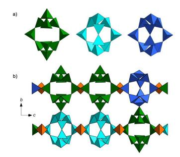
**Figure 3.** (a) Cages of type 1 (green), type 2 (turquoise), and type 3 (blue). (b) Repeating unit in  $[Si_{22}O_{19}N_{36}]^{58-}$  layers, viewing direction [100].
