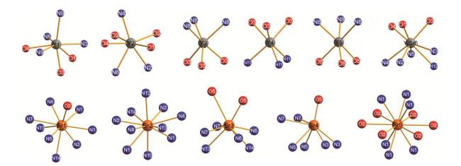
Figure S4. Coordination spheres of Y, Y/Sr, and Sr sites.
