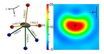
**Figure 5.** Left: Coordination sphere around Y39 with long green and significantly shorter yellow distances. Right: Resulting electron density distribution ( $F_{obs} - F_{calc}$ ) with viewing direction along the Y39–O47 bond (scale bar in  $e^{-}/a_{0}^{3}$  with  $a_{0}$ : Bohr radius).<sup>[40]</sup>
