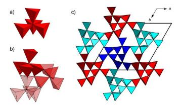
**Figure 2.** (a) Star-shaped  $[C^{[4]}(Si(O/N)_3)_4]$  unit. (b) Entity of three condensed  $[C^{[4]}(Si(O/N)_3)_4]$  units. (c) Anionic  $[Si_{12}O_2N_{16}C_3]^{16^-}$  network built up of entities from (b). The blue and turquoise entities are distorted variants of the red entity.
