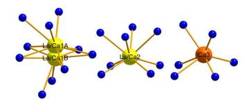
**Figure 3.** Coordination spheres of the heavy atom sites in  $La_{3-x}Ca_{1.5x}Si_6N_{11}:Eu^{2+}$ . Mixed occupied La/Ca sites are yellow, Ca orange, and N atoms blue.
