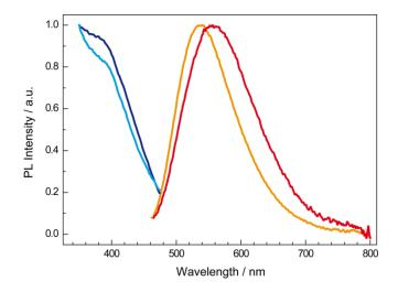
**Figure 5.**  $Lu_4Ba_2[Si_{12}O_2N_{16}C_3]:Eu^{2+}$ : normalized excitation spectrum (550–570 nm) dark blue, emission spectrum ( $\lambda_{exc} = 440$  nm) orange;  $Y_4Ba_2[Si_{12}O_2N_{16}C_3]:Eu^{2+}$ : normalized excitation spectrum ( $\lambda_{mon} = 570-610$  nm) cyan, normalized emission spectrum ( $\lambda_{exc} = 440$  nm) red.
