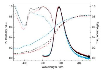
**Figure 6.** Excitation (dotted line), emission (line), and diffuse reflectance (dashed line) spectra of  $La_{3-x}Ca_{1.5x}Si_6N_{11}$ :  $Eu^{2+}$  ( $x \approx 0.77$ ) for varying Eu concentrations (1 mol%: cyan; 2 mol%: black; 4 mol%: red).
