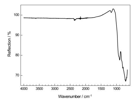
**Figure S6.** ATR-FTIR spectrum of a  $Y_4Ba_2[Si_{12}O_2N_{16}C_3]:Eu^{2+}$  powder sample. Bands at 2345 cm<sup>-1</sup> belong to the asymmetric stretching vibration of CO<sub>2</sub>. No O–H and N–H bands are observed in the typical region.
