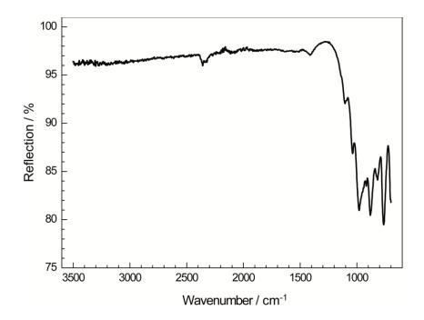
**Figure S2.** ATR-FTIR spectrum of a  $Y_{23}Sr_{17}[Si_{38}O_{18}N_{67}]O_9$  powder sample. No N-H and O-H bands are observed in the typical region.
