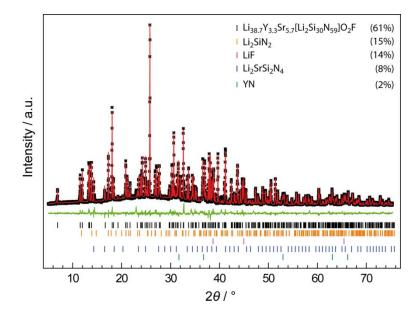
**Figure S14.** Rietveld refinement of data collected from a  $Li_{38.7}Y_{3.3}Sr_{5.7}[Li_2Si_{30}N_{59}]O_2F$  sample ( $\lambda = 1.54056$  Å). Experimental PXRD data as black stars, Rietveld fit red, difference plot green. Reflection positions of  $Li_{38.7}Y_{3.3}Sr_{5.7}[Li_2Si_{30}N_{59}]O_2F$  as black bars. The sample also contains  $Li_2SiN_2$  (orange bars, 15 wt%), LiF (magenta bars, 14 wt%),  $Li_2SrSi_2N_4$  (blue bars, 8 wt%), and YN (green bars, 2 wt%).
