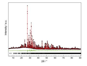
Figure 1. Rietveld refinement for washed  $Y_{26}Ba_6[Si_{22}O_{19}N_{36}]O_{16}$ : Eu<sup>2+</sup> (Cu K $\alpha_1$ ,  $\lambda$  = 1.54056 Å).
