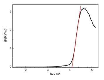
Figure 5. Tauc plot (n = 1/2) for nondoped Li<sub>38.7</sub>La<sub>3.3</sub>Ca<sub>5.7</sub>[Li<sub>2</sub>Si<sub>30</sub>N<sub>59</sub>]O<sub>2</sub>F.
