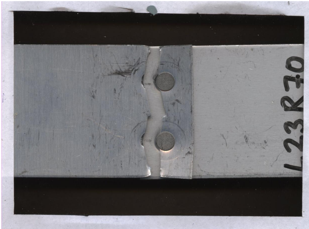
Figure 17: Eyebrow failure at maximum load of 3 KN at 1.54 million cycles
