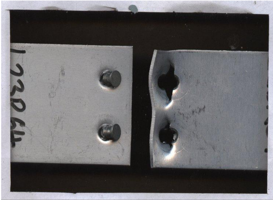
Figure 23: 3-9 failure at maximum load 8 KN at 51000 cycles
