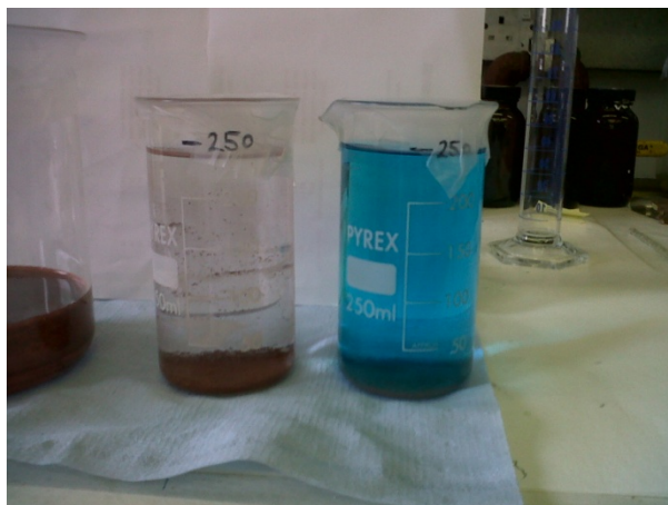
Figure (51) Effect of ultrasound on the electroless copper bath
