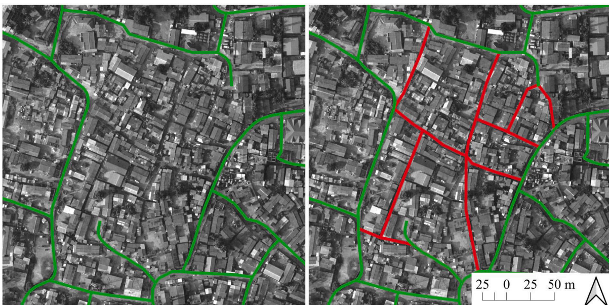
Fig. 1. Increasing data coverage in Akweteman. In green, the original OSM street network. In red, the added streets. (For interpretation of the references to colour in this figure legend, the reader is referred to the web version of this article.)
