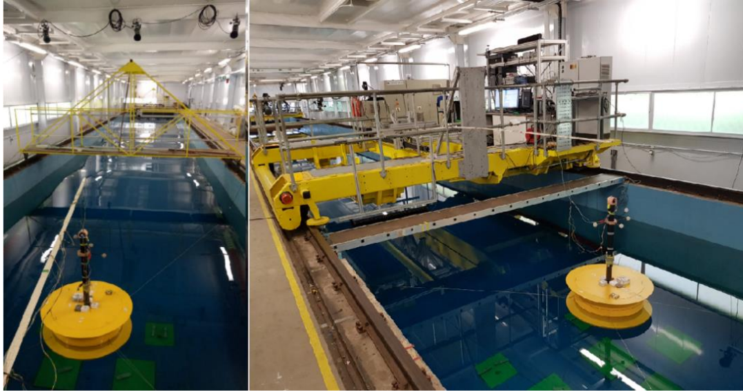
Figure 7: Qualisys camera system attached in the tank roof and the model moored at tank centre in front of carriage.
