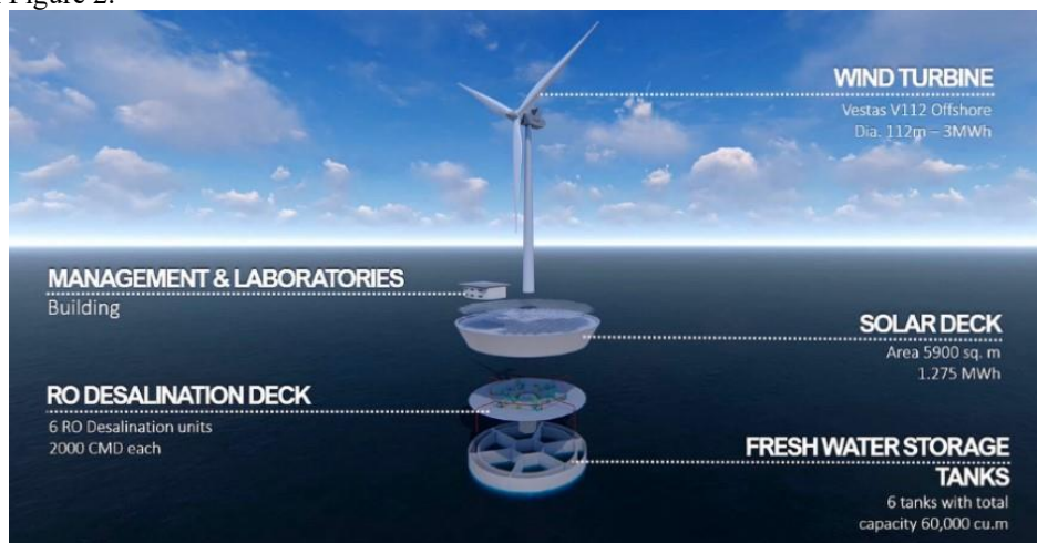
Figure 2: Proposed floating desalination plant concept.
