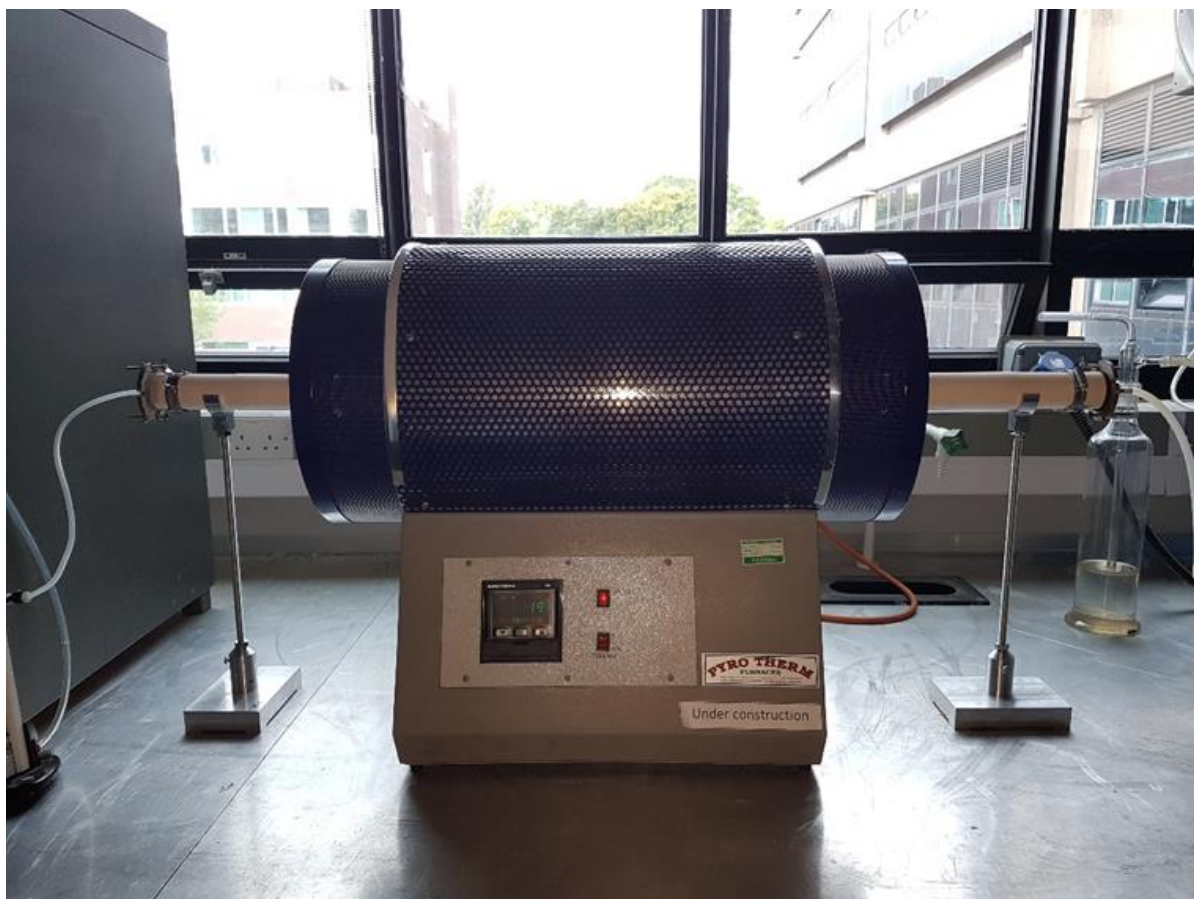
Figure 3.5 The furnace assembly used for the heat treatment of lignin fibres.
