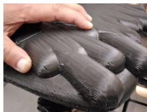
Figure 10. Aesthetic effect of 3D printed hatches for surface filling (seat of Flamingo chair).
