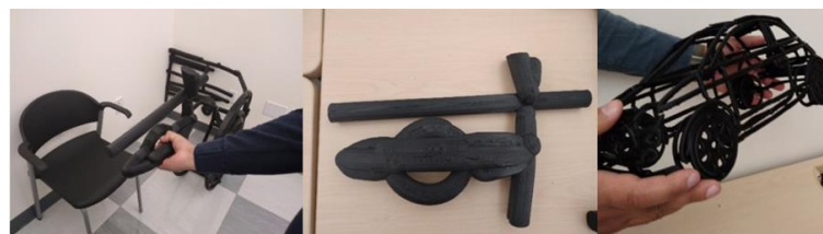
Figure 8. Car door handle (partial) 3D printed at real scale (the chair shows the scale) (left-center), manipulating and touching the model (left).
