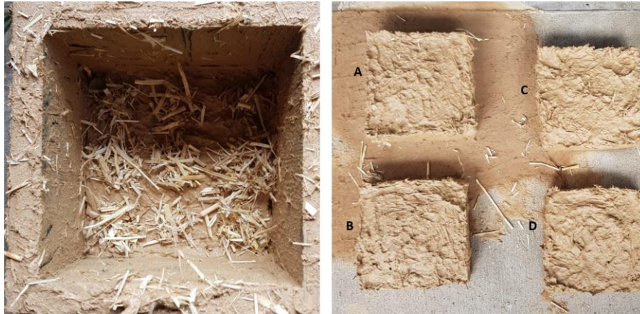
Figure 10. (left): Mud block C: straw pocketing; (right): Mud block A- the control that has no straw density grid layer; Mud block B- 1 layer of the straw density grid using medium length fibers at \frac{1}{2} ; Mud block C- 1 layer of the straw density grid using short length fibers at \frac{1}{2} ; Mud block D- 2 layers of straw using short fibers at \frac{1}{3} and \frac{2}{3} .
