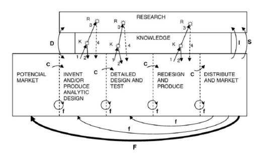
Chain-linked model showing flow paths of information and cooperation. Symbols on arrows:  $\mathbf{C} = \text{central-chain-of-innovation}$ ;  $\mathbf{f} = \text{feedback loops}$ ;  $\mathbf{F} = \text{particularly important feedback}$ .
