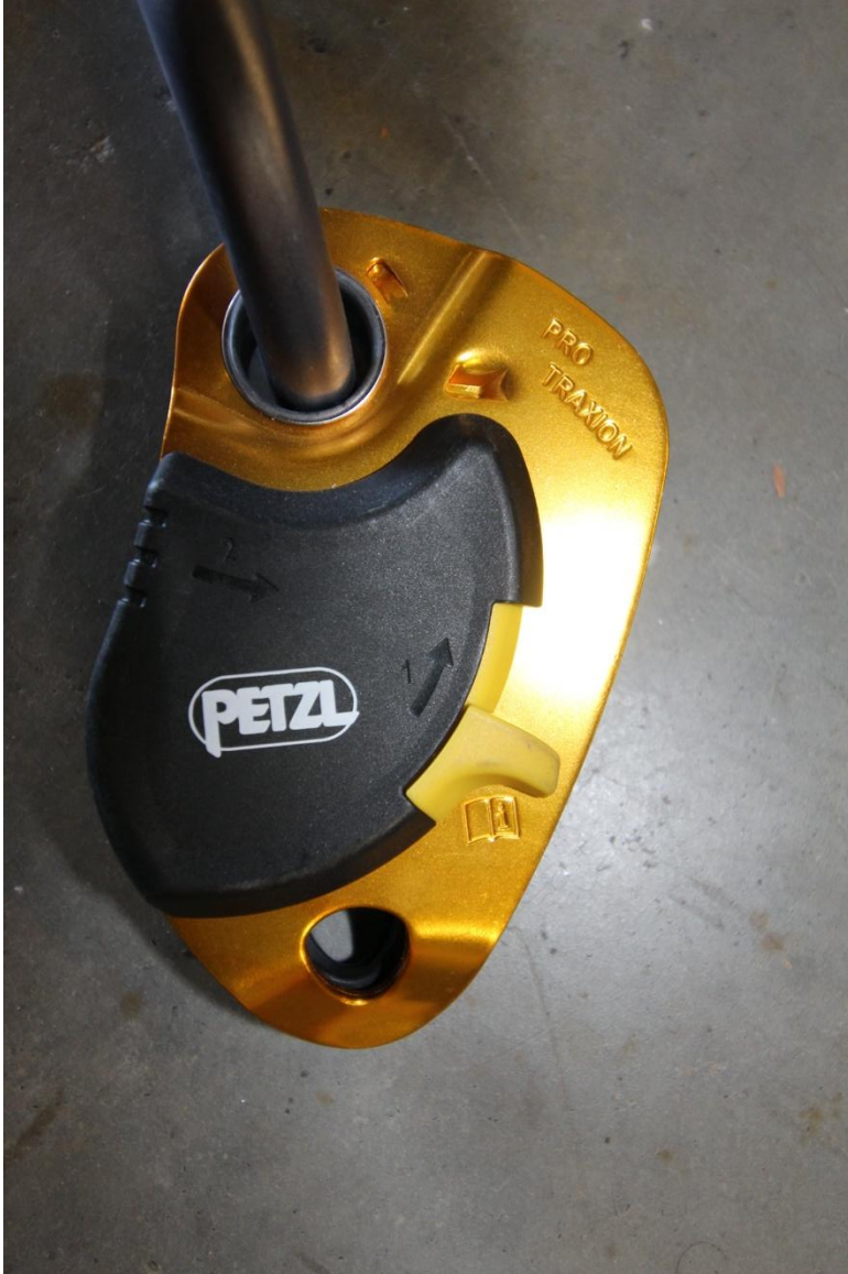
Image 12 – Pro Traxion (Progressive Capture Single Pulley)
