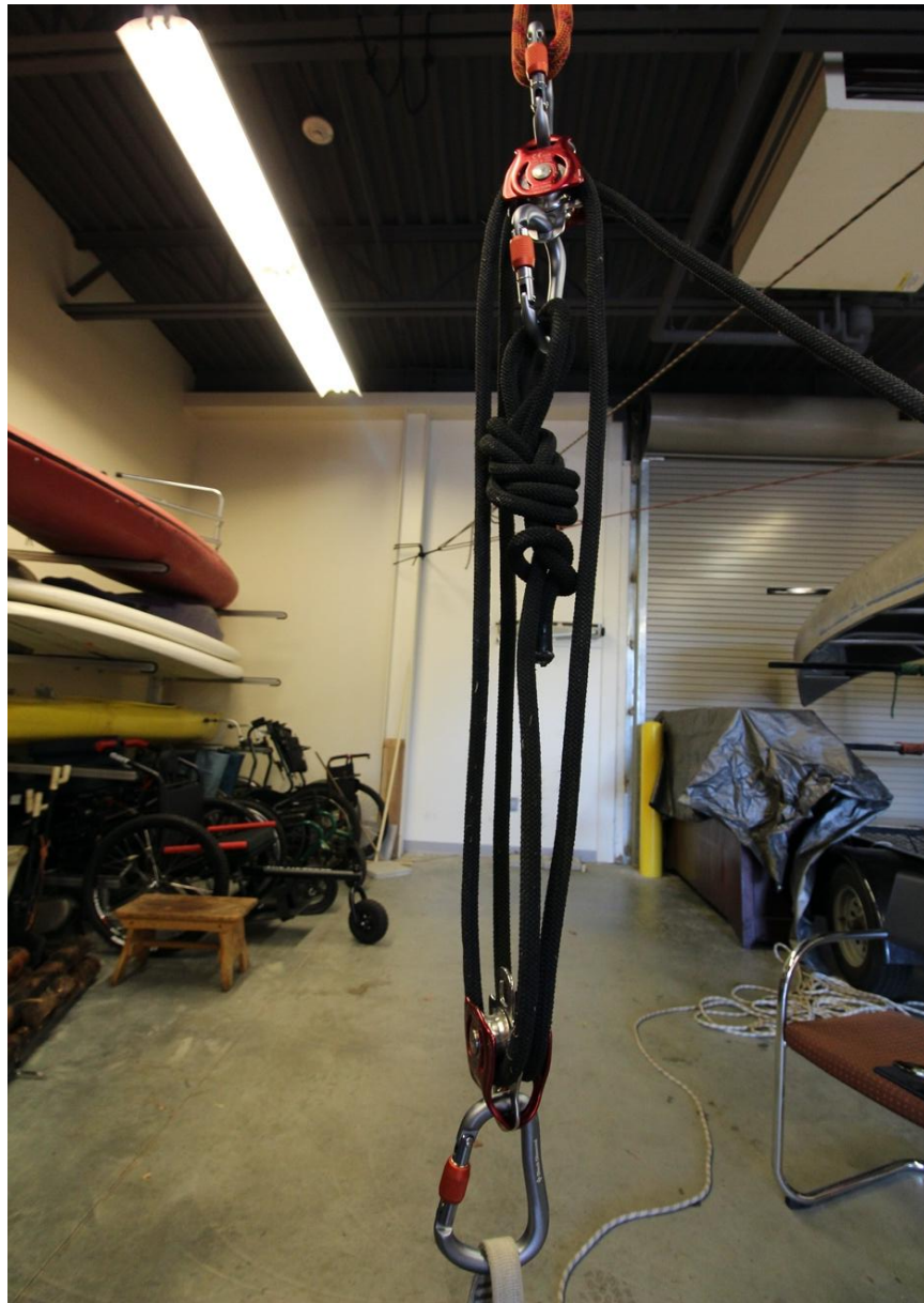
Image 17 - 4:1 Mechanical Advantage System
