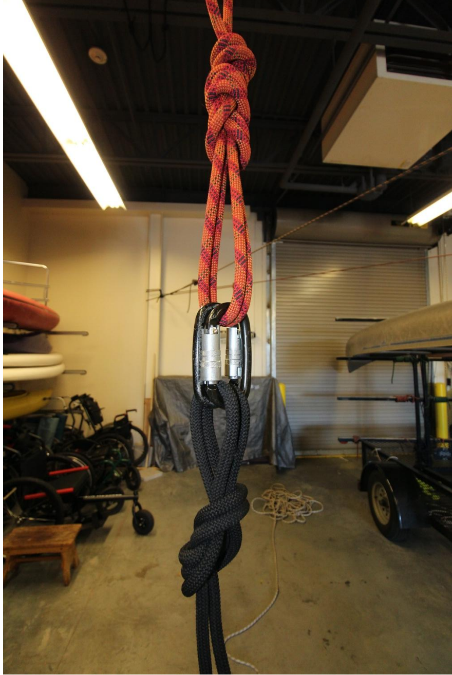
Image 13 - 1:1 Basic Ascending (NOT a Mechanical Advantage System)
