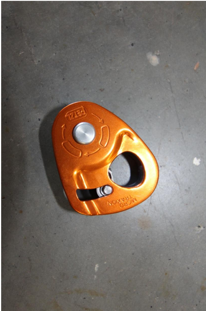
Image 11 – Micro Traxion (Progressive Capture Single Pulley)
