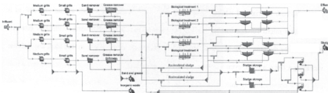
Fig. 3. Modeling the technological configuration of the wastewater treatment process currently used in Timisoara Wastewater Treatment Plant, using BioWin software suite
