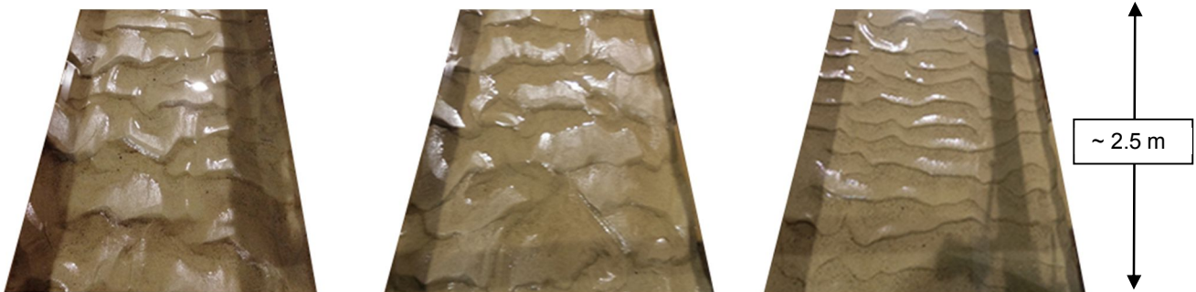
Figure 4. Photos of the bedforms obtained in Runs 1, 2 and 3. Flow from top to bottom.
