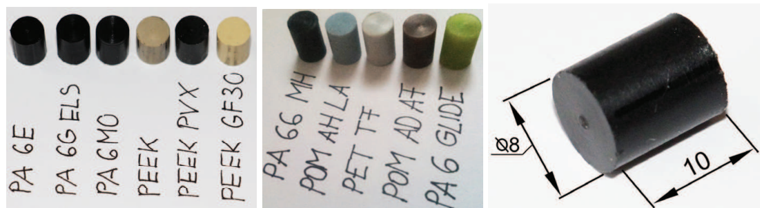
Figure 2. Original form and dimensions of the tested polymers and composites.
