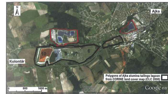
Figure 3 – Polygons of the mine waste sites defined from the CORINE land cover map (CLC 2000) overlaid by Google Earth® aerial photographs (2010-2011) to answer EU Pre-selection Protocol questions Q13-14 on the air and direct contact pathways related to the cover of tailings. Example shows the Ajka alumina plant tailings lagoon. Note that cells 9 and 10 are not covered while cells 1-8 have been rehabilitated with soil and plant cover
