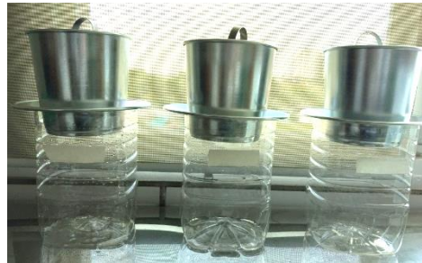
Figure 2. Coffee filters were used for measuring the water holding content and soil moisture
