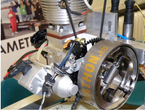
Figure 6: Setup for measuring the instantaneous torque
