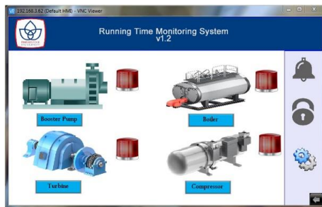
Figure 13. The HMI's main screen via laptop/PC
