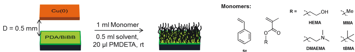
Figure 4.3: Schematic illustration of the synthesis of polymer brushes on PDA/BiBB via SI-CuCRP. A Cu(0)-surface is clamped at a distance D = 0.5 mm over the PDA/BiBB substrate and the assembly is immersed into degassed reaction solution.
