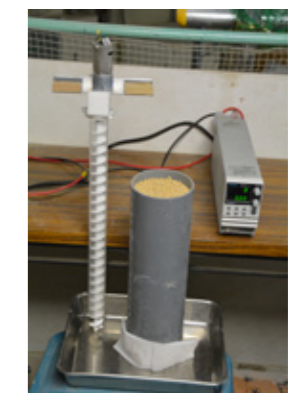
Fig.6 Auger screw-type soil sampling device
