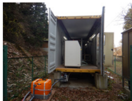
Fig.3 Field test of binary power plant for hot springs
