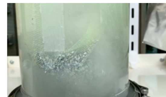
Fig.5 H 2 production (bubbles) using waste Al chips and Tamagawa hot spring water
