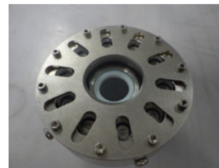
Fig.6 Scanning head of borehole scanner for geothermal well
