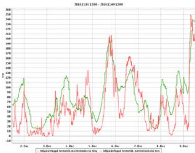
Illustration 10: The time table (green line) and the real production (red line) which shows suitable correspondence in case of 0-85% change in production for an interval of seven days.
