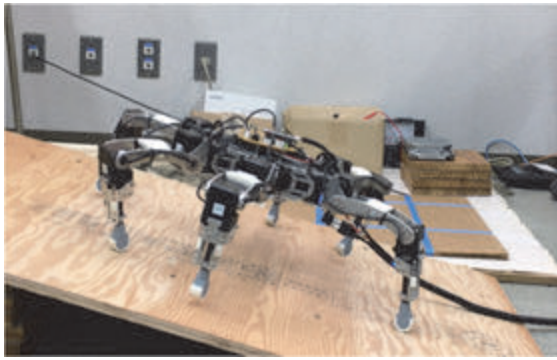
Fig. 18 Walking experiment on slope road course without posture control
