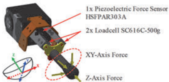
Fig. 2 Placement of sensors and hemisphere sensing range
