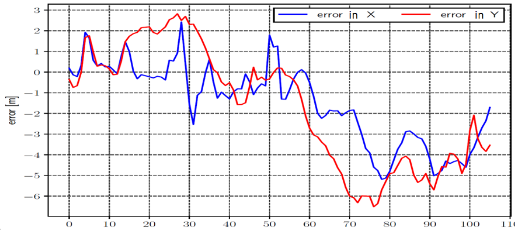
Fig. 9. a) Some images obtained from the drone's point of view when performing this trajectory; b) trajectory in open field estimated by EVP in blue, and ground truth obtained from GPS-RTK in red; c) Trajectory error vs. number of measures over time
