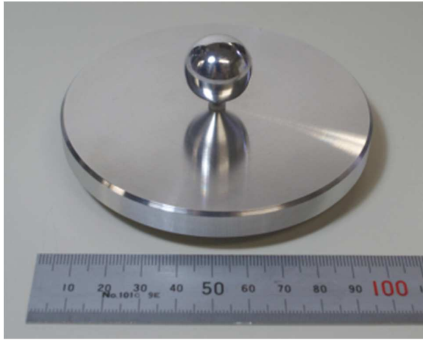
Fig. 2.15. Antenna under test: low-VSWR monopole antennas [44].
