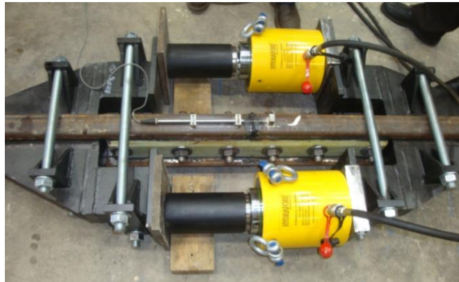
Fig. 3 Test set-up of axial pulling test
