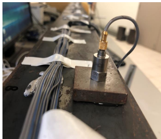
Figure 6-4: Strain gauge and accelerometer - Underneath the beam
