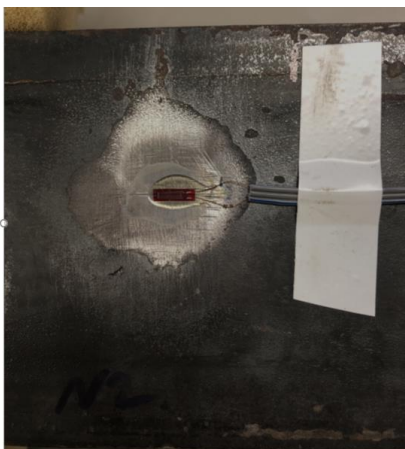
Figure 6-4: Strain gauge and accelerometer - Underneath the beam
