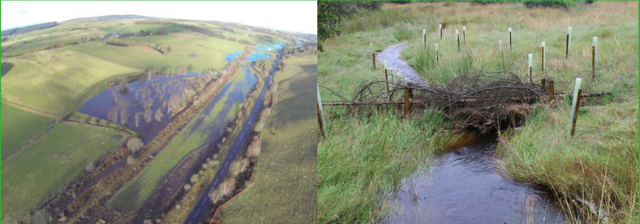
Figure 2: Eddleston Water Project Natural-Flood Management Measures (left, aerial photo © Tweed Forum; right, log jam © Chris Spray)
