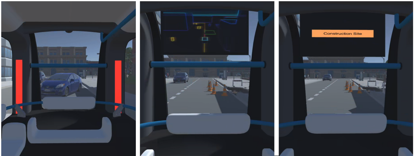
Figure 1: Three out of the five designed modalities. Left: reactive critical - light, middle: proactive non-critical - visualisation, right: proactive non-critical - text.
