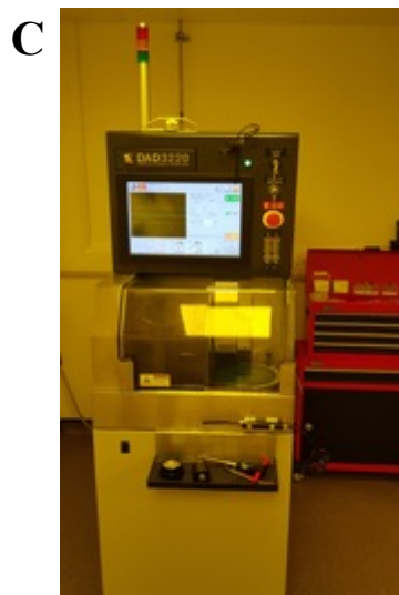
Figure 2.5: Equipment used for photolithography. (A) Spin coater for applying layer of either positive or negative photoresist onto borosilicate. (B) Photomask aligner for aligning film photomask over photoresist coated borosilicate and for UV exposure. (C) Dicing saw used for cutting borosilicate to measure 49 x 49 mm. (D) Laser lithography system for etching array design into photoresist without the requirement of a photomask.
